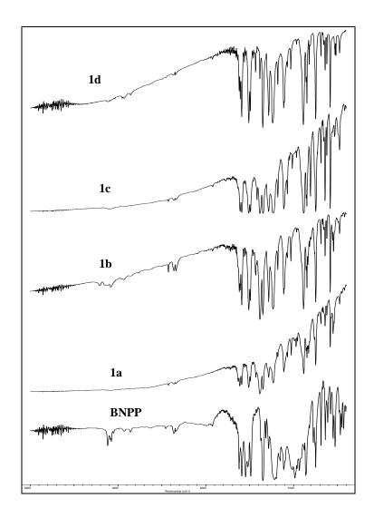
FT-IR spectra of **BNPP** and the complexes **1a**, **1b**, **1c** and **1d** recorded in KBr.
