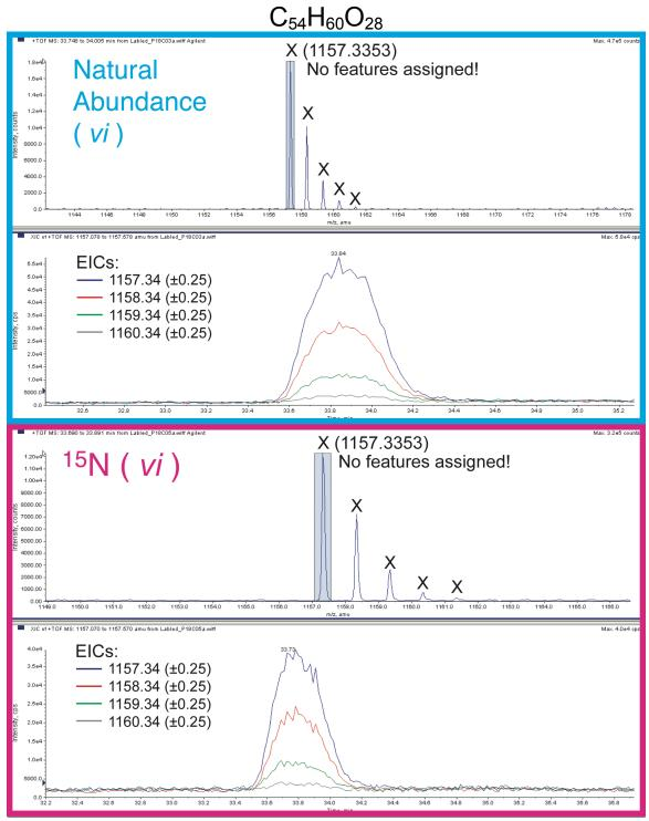
• This example is a clear failure to assign <u>any</u> features to this species. It is well separated chromatographically and so manual assignment was trivial.
