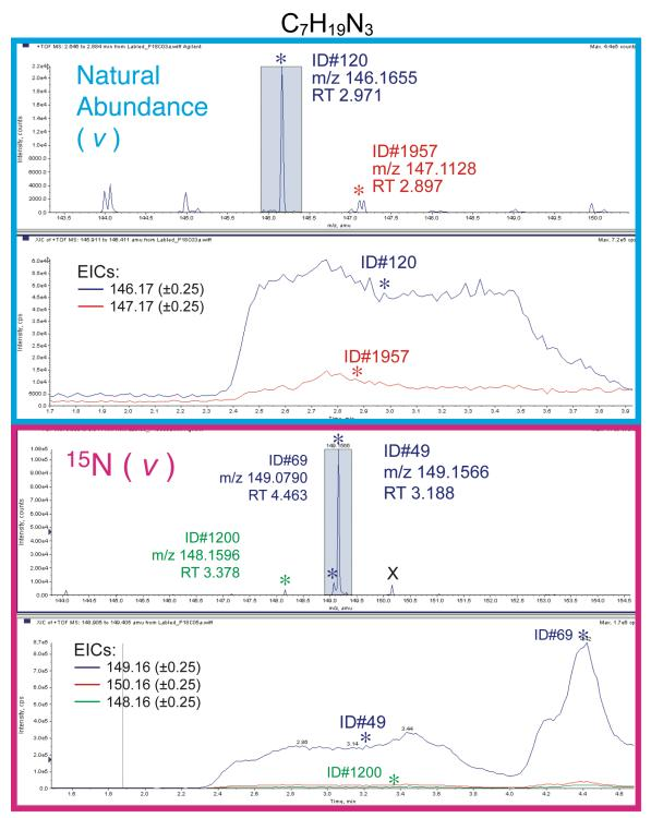
• This is a compound eluting in the flow through. The peak shape is terrible and there are lots of coeluting species suppressing ionization and overlapping in the spectra. Features are assigned within non-ideal elution profiles.
