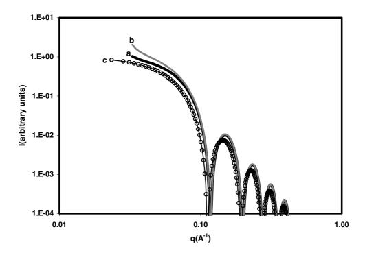
**Figure 1:** Radial averages including step by step the different effects. The P(q) of a pure sphere has been taken as the exact solution (curve c)to be retrieved. Curve a: taking no correction into account; curve b: taking only absorption into account ; curve c: taking absorption and refraction into account.
