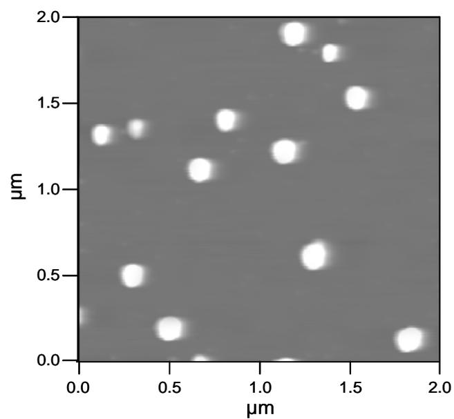
**Figure S2.** AC mode AFM height image of 45 mol% AHAP3 silica nanoparticles (balance TEOS) on a mica surface.
