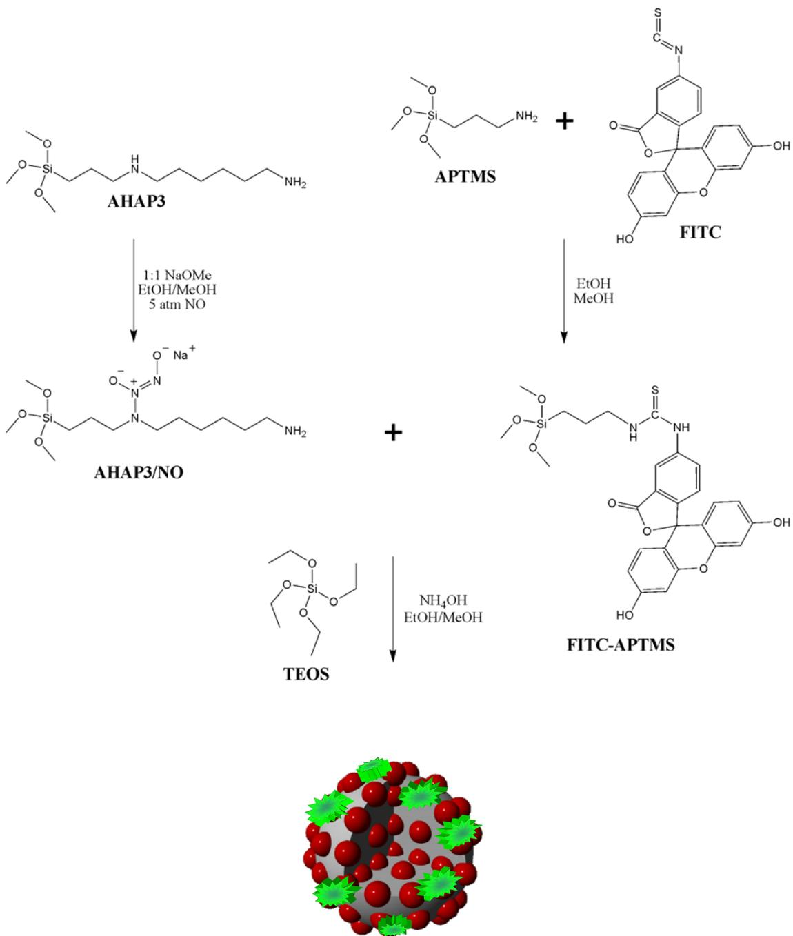
**Scheme S1.** Synthesis of FITC-modified NO-releasing 45 mol% AHAP3 silica nanoparticles (balance TEOS). Abbreviations: AHAP3 =  $N$ -(6-aminohexyl)aminopropyltrimethoxysilane; APTMS = 3-aminopropyltrimethoxysilane; FITC = fluorescein isothiocyanate; TEOS = tetraethoxysilane.
