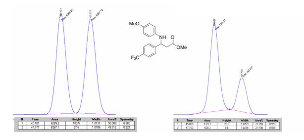
HPLC analysis using CHIRALCEL OD-RH column (45:55 CH<sub>3</sub>CN-H<sub>2</sub>O).
