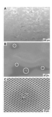
Figure 3S: A-B) SEM images of posts etched in silicon using the negative resist and same photomask. These images illustrate that all surfaces are less rough than those with the nm-tips.
