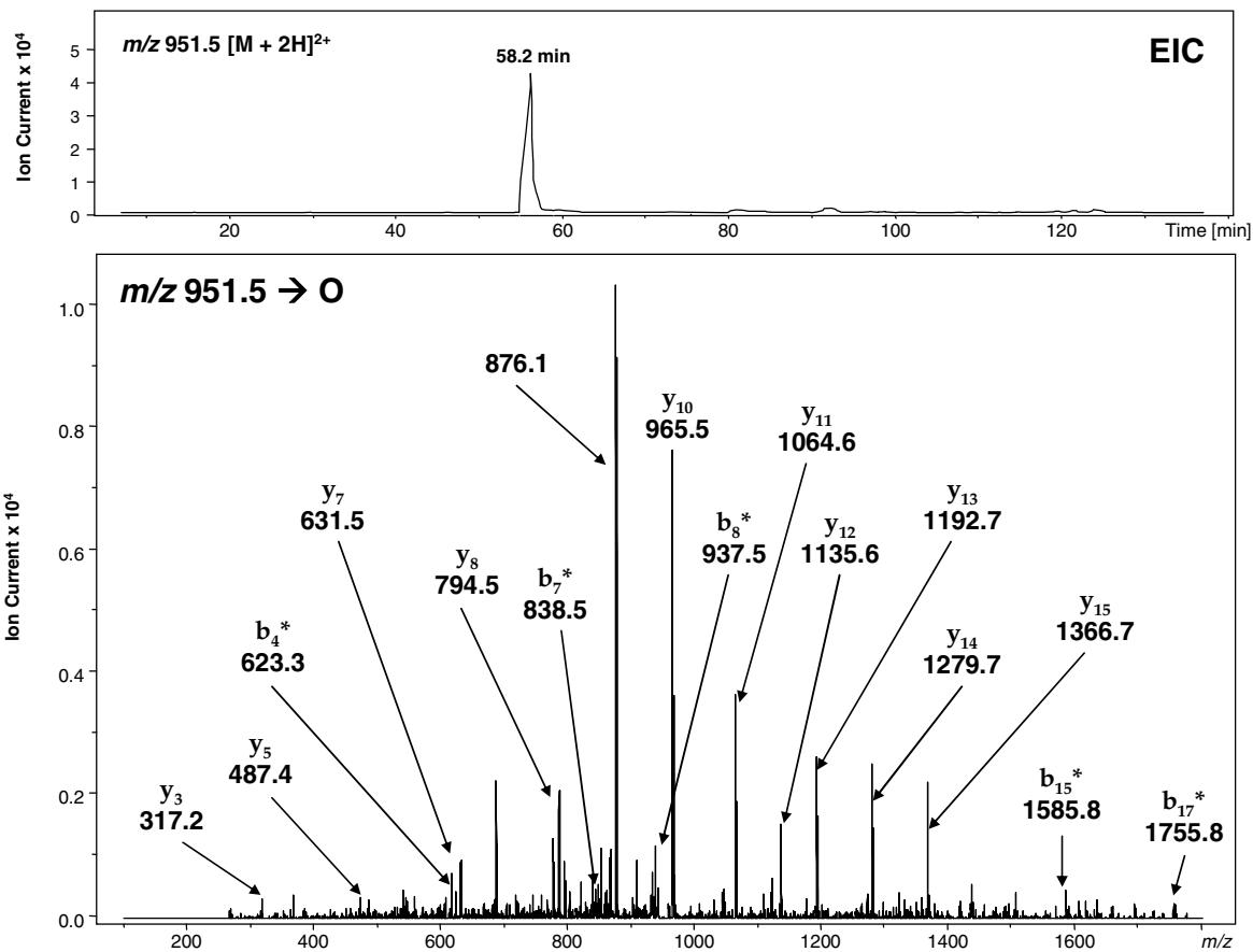
**S-9.** HPLC-ESI<sup>+</sup>-MS/MS analysis of AGT tryptic peptides G<sup>136</sup>NPVPILIPCHR<sup>147</sup> (**A**) and V<sup>148</sup>VCSSGAVGNYSGGLAVK<sup>165</sup> (**B**) containing chlorambucil cross-links to guanine obtained from chlorambucil treatments of AGT-DNA mixtures.
