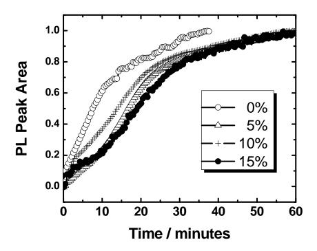
**Figure S1**: Photoluminescent peak area evolution of core-shell quantum dots during  $\sim$ 1 hr of ZnS shell growth. The presence of In<sup>3+</sup> does not significantly alter the rate of ZnS shell growth.
