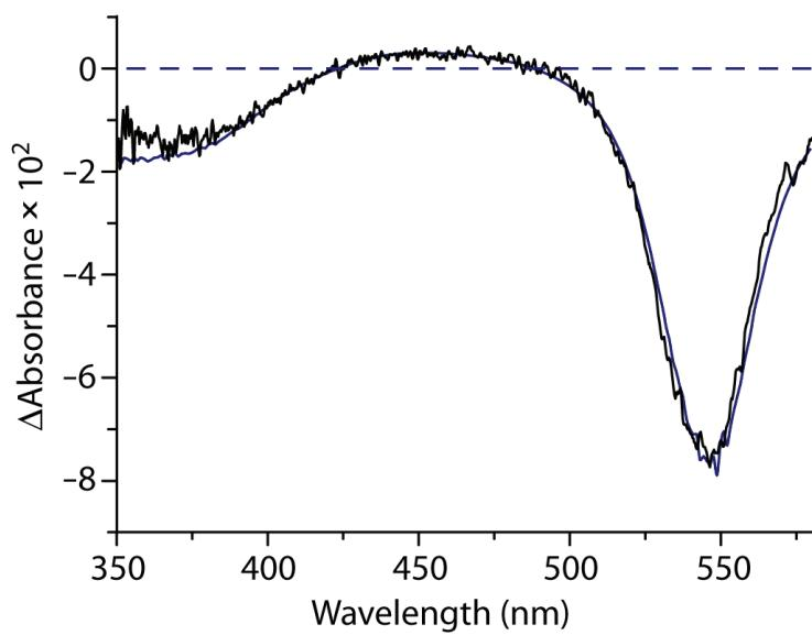
**Figure S12.** (black) Transient absorbance UV-Vis spectrum observed at of **2** following excitation with a 10 ns laser pulse. (blue) The spectrum that results from digital subtraction the spectrum of **2** from the spectrum of the mixture of products formed during exhaustive photolysis at 546 nm. These spectra are shown in figure 11 of the main text.
