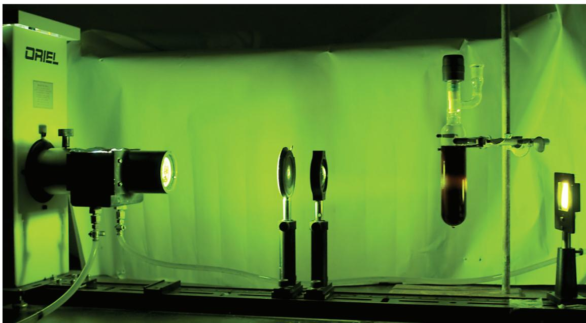
**Figure S22.** Table of Contents Graphic: This photograph shows the photochemical bleach of **2** when irradiated by an Oriel 1000 W Hg-Xe arc lamp equipped with a  $\lambda \geq 480$  nm filter. The area above and below the bleach are still purple because these areas were not directly in the beam of light. The backstop is illuminated upon completion of the photochemical bleach when light at this wavelength is no longer absorbed by the solution.
