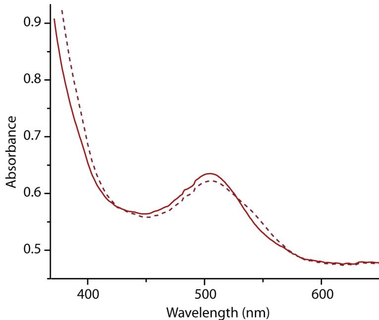
**Figure S11.** UV-Vis spectrum of **2**<sup>2+</sup> (—) taken in an optically transparent thin-layer electrode at a potential difference of -50 mV, and of electrochemically generated **2**<sup>+</sup> (- - -) holding the solution at a potential of -750 mV. This experiment was carried out in 0.5 M [(n-Bu)<sub>4</sub>N][PF<sub>6</sub>]/THF at 20 °C.
