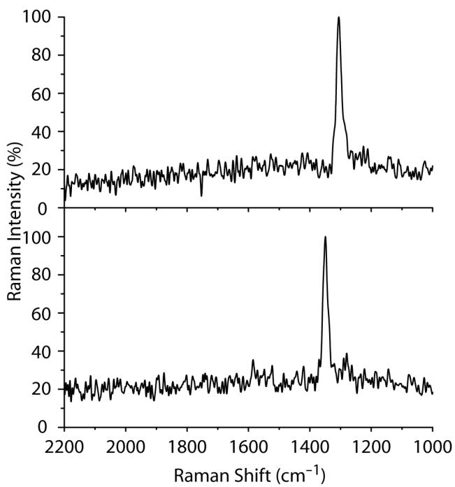
**Figure S7.** Resonance Raman spectra ( $\lambda_{\text{excite}} = 514.5 \text{ nm}$ ) of  $\mathbf{2}[\text{B}(\text{Ar}^{\text{F}})_4]_2$  in  $\text{CH}_2\text{Cl}_2$ .
