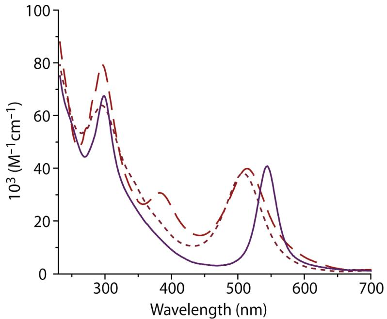
**Figure S10.** Electronic absorption spectra for **2** (—) in  $\text{Et}_2\text{O}$ , **2** $[\text{B}(\text{Ar}^{\text{F}})_4]$  (- - -) in  $\text{CH}_2\text{Cl}_2$ , and **2** $[\text{B}(\text{Ar}^{\text{F}})_4]_2$  (—) in  $\text{CH}_2\text{Cl}_2$  are shown 20 °C.
