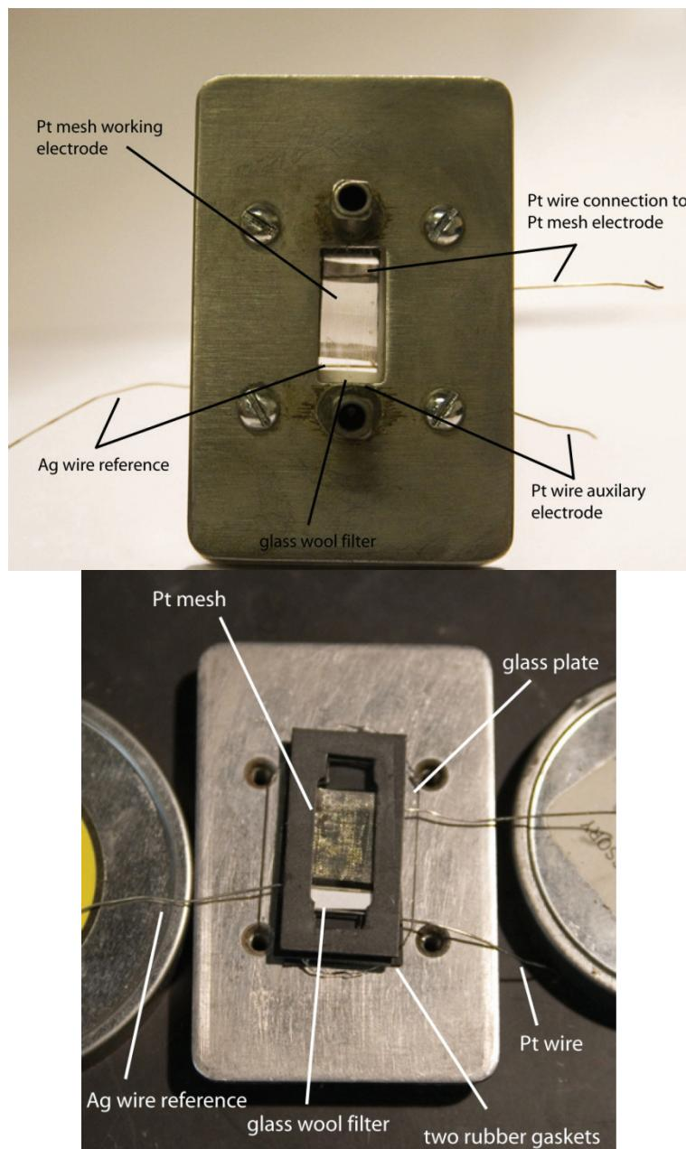
**Figure S23.** An optically transparent thin-layer electrode (OTTLE) constructed from a solution IR spectroscopy cell is suitable for the study of air-sensitive compounds. This electrochemical cell is adapted from literature designs.<sup>32,33</sup>
