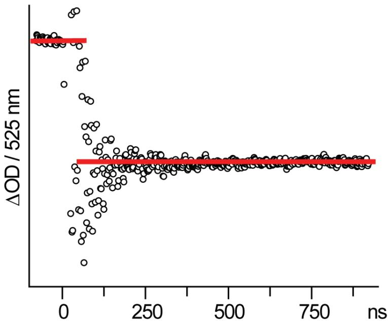
**Figure S13.** The kinetics of photochemical NN bond cleavage of **2** are shown on a ns timescale. The data points correspond to changes in absorbance measured at 530 nm with time. The line to guide-the-eye is a step function indicating that the photochemical process is faster than the resolved timescale.
