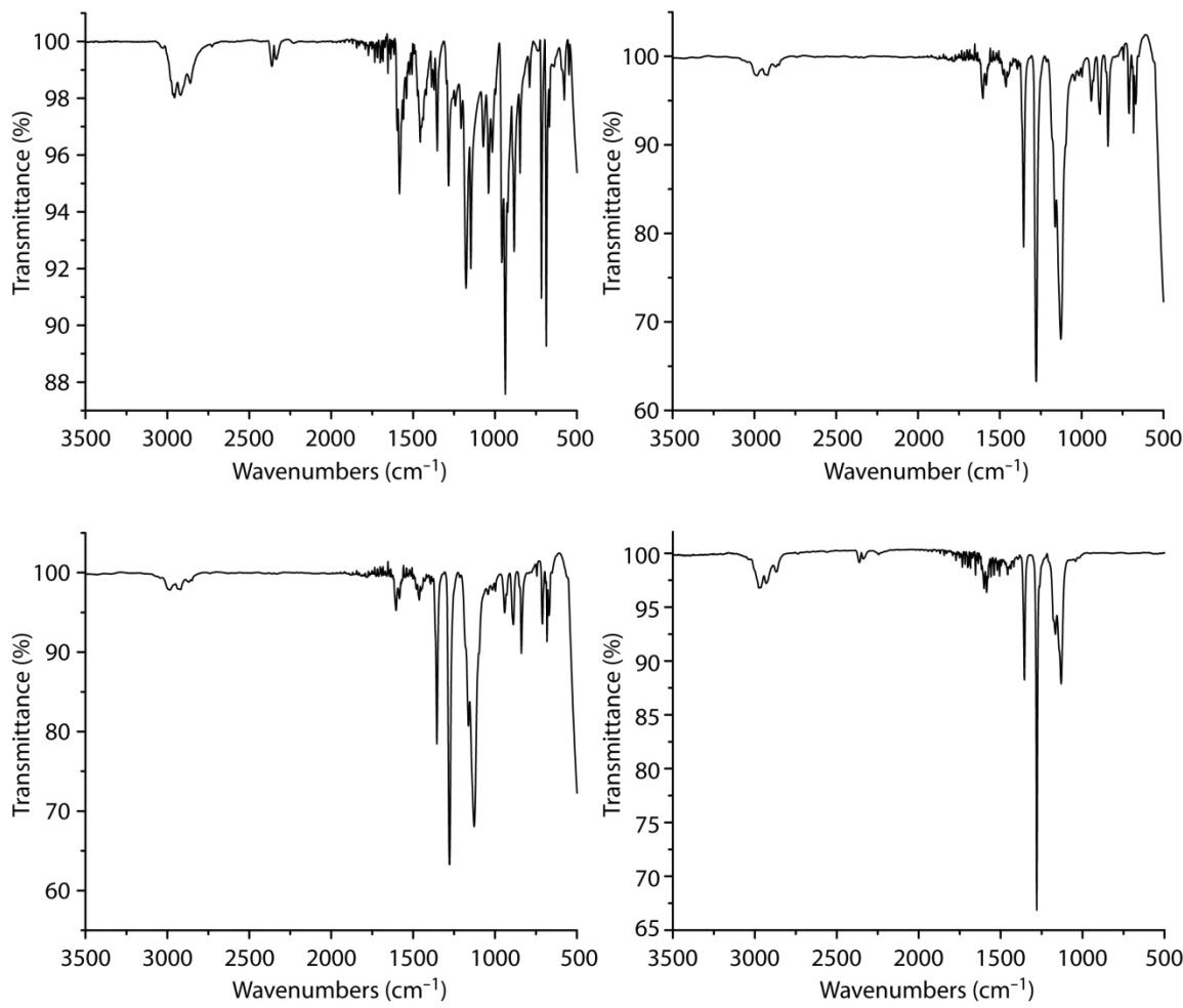
**Figure S9.** Infrared spectra as thin films (KBr) of **2** (top-left), **2[B(Ar<sup>F</sup>)<sub>4</sub>]<sub>2</sub>** (top-right), **2[B(Ar<sup>F</sup>)<sub>4</sub>]** (bottom-left); and **2[B(Ar<sup>F</sup>)<sub>4</sub>]** in CDCl<sub>3</sub> (bottom-right). Note that the Raman active  $\nu_{NN}$  is not detected in the infrared spectrum for any of these three molecules.
