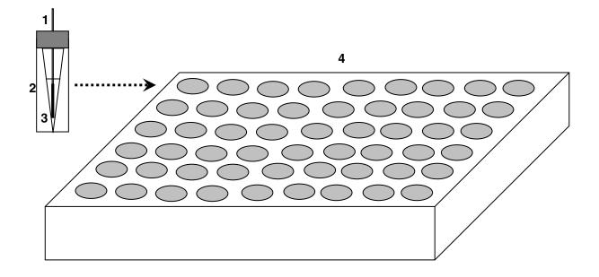
Figure S1. Desorption device for *in vivo* and field sampling: (1) SPME fiber, (2) 2mL vial, (3) 200-µL insert, and (4) 54-vial plate.
