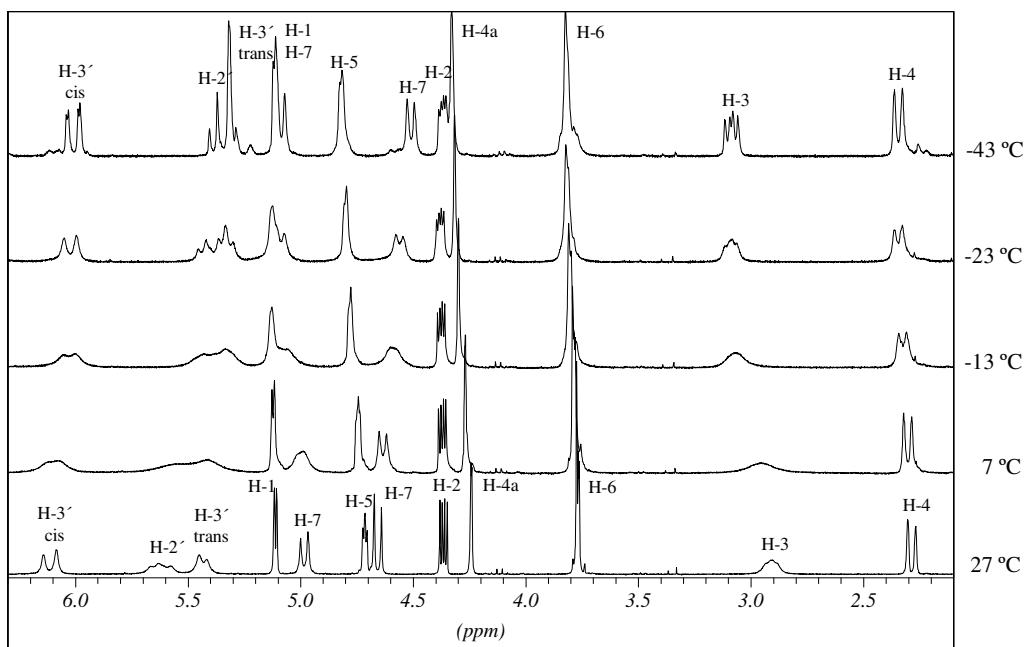
$^1\text{H}$  NMR (300 MHz,  $\text{CDCl}_3$ ) Spectra of **6** with  $\text{Et}_2\text{AlCl}$  recorded at 300 K
