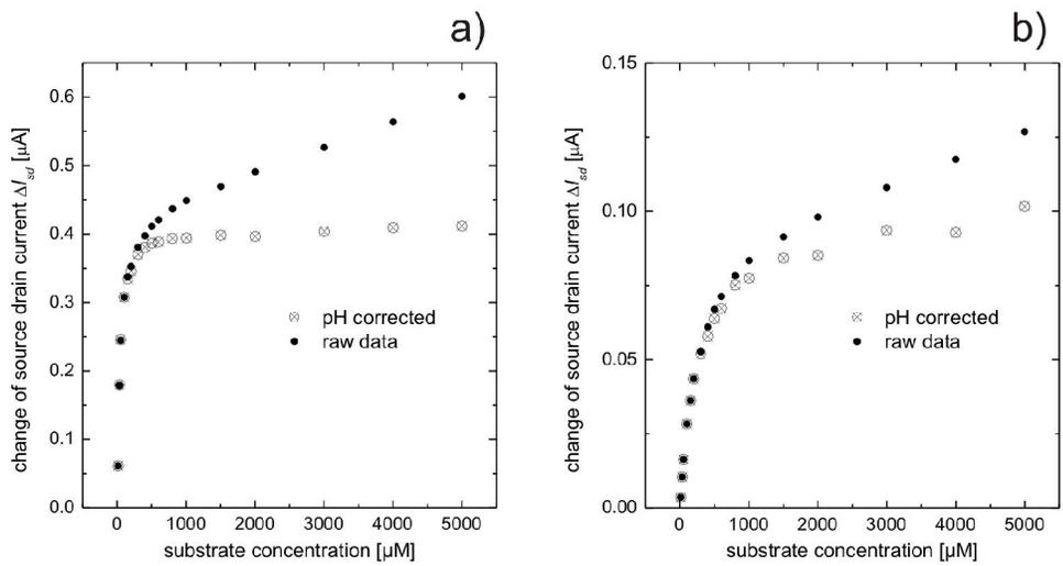
Variation of the source-drain-current  $I_{sd}$  as a function of acetylcholine chloride. The graphs compare the raw data and pH corrected data for the AchE-EnFET in the case of standard and diluted (1:10) buffer solutions, right and left graphs, respectively. The pH correction mainly affects the saturation region in the case of measurements using a diluted buffer.
