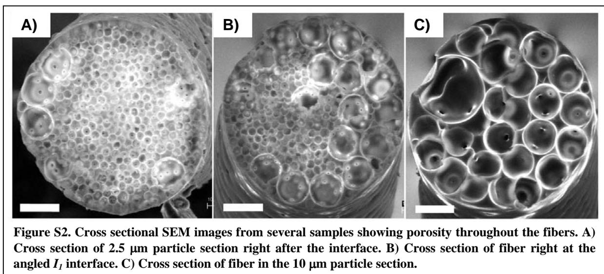
Figure S2 depicts cross sectional SEM views of different sections/interfaces taken from several fibers. The images clearly show that the fibers are porous throughout the fiber cross section. The samples are prepared for cross sectional analysis by dipping the fibers into liquid  $N_2$  and subsequent pulling until the fiber breaks.
