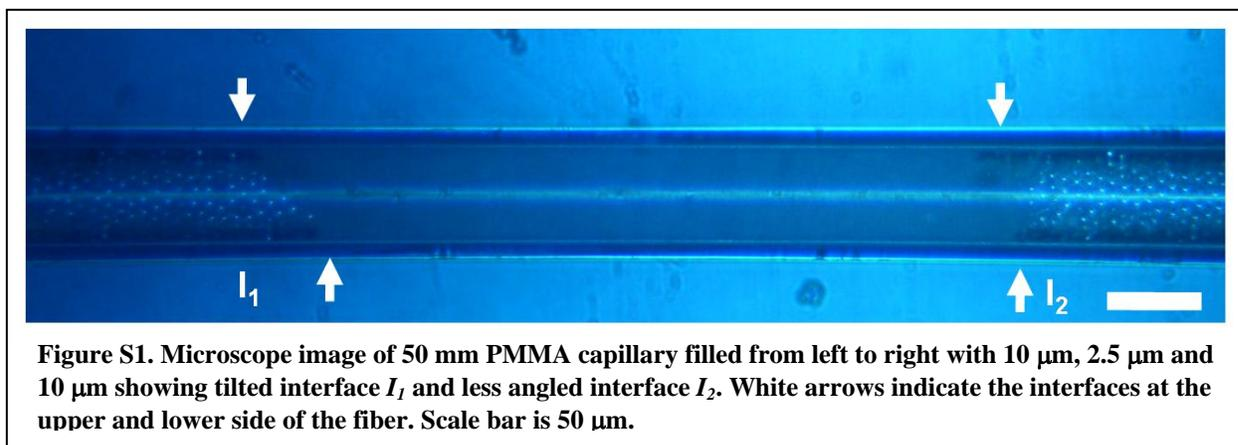
Figure S1 shows a microscope image of the two interfaces  $I_1$  and  $I_2$  produced during alternating colloidal assembly of 10 μm, 2.5 μm, and 10 μm colloids within a 50 μm PMMA capillary. The strongly tilted angle of the  $I_1$  interface caused by sedimentation of the 10 μm particles is clearly visible.  $I_2$  is much less tilted.
