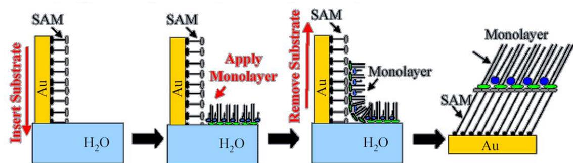
Figure 1. Schematic of the process of LB film deposition
