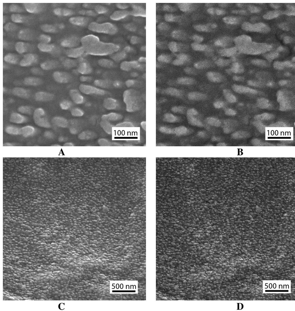
**Figure S20.** SEM images of composite **C1** (A, C: secondary electron images, B, D: backscattered electron images). The surface was cryo-microtomed, stained by 0.5%  $\text{RuO}_4$  solution vapor for 30 min, and then coated with ~2 nm of Pt by direct Pt sputtering.
