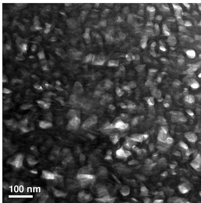
**Figure S22.** TEM image of composite **C1**. The thin film was stained by 4% OsO<sub>4</sub> solution vapor for 15 min before imaging.
