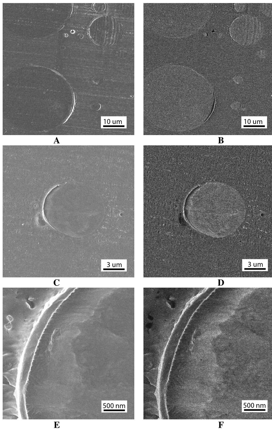
**Figure S21.** SEM images of composite **C2** (A, C, E: secondary electron images, B, D, F: backscattered electron images). The surface was cryo-microtomed, stained by 0.5% RuO<sub>4</sub> solution vapor for 30 min, and then coated with ~2 nm of Pt by direct Pt sputtering.
