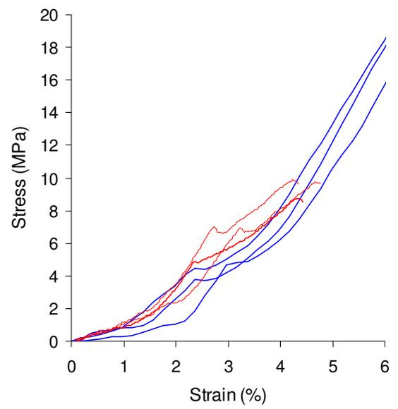
**Figure S24.** Tensile tests on composite **C1** (blue) and **C2** (red).
