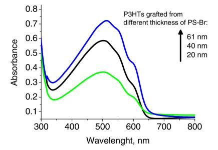
Figure S2. UV-spectra of grafted P3HT brushes from different thicknesses of PS-Br
