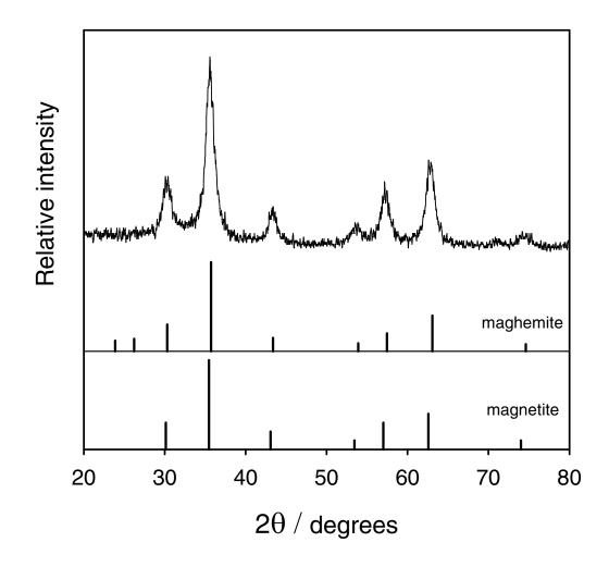
**Figure 1.** X-ray diffraction pattern of synthetized iron oxide nanoparticles compared to literature data3 for maghemite ( $\gamma$ -Fe<sub>2</sub>O<sub>3</sub>) and magnetite (Fe<sub>3</sub>O<sub>4</sub>).
