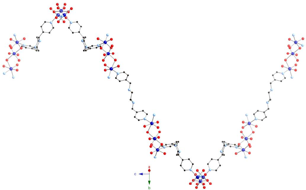
Figure S4. Quartz (**qtz**) net formed from junction of *helix-1* and *helix-2* motifs.
