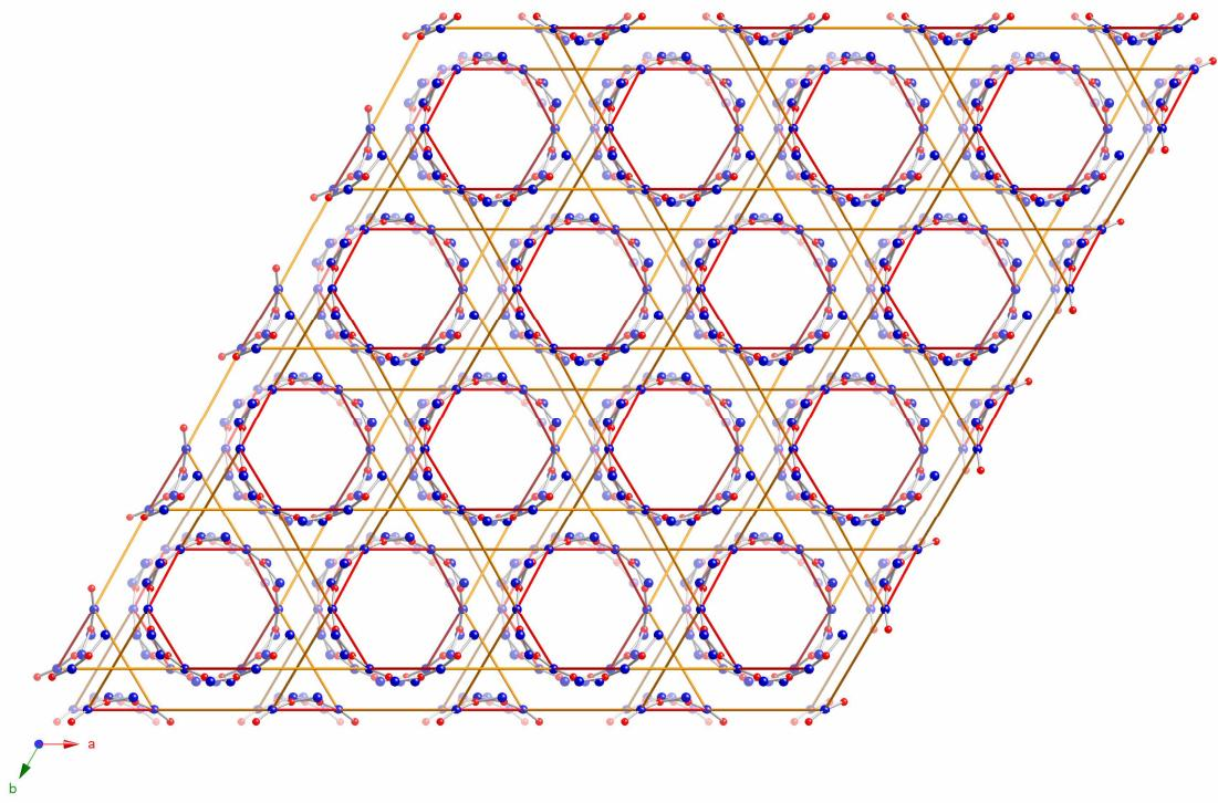
Figure S5. Quartz (**qtz**) net formed from junction of *helix-1* and *helix-3* motifs.
