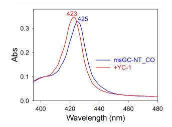
UV-visible spectra of the msGC-NT-CO Soret band  $\pm$  YC-1. Note the 2 nm shift in, and sharpening of, the band in the presence of YC-1. BAY 41-2272 (not shown) induces a similar change in the spectrum.
