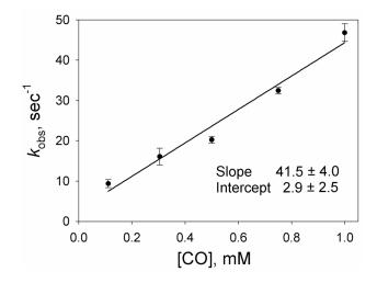
Dependence of  $k_{obs}$  on CO concentration for the slower photolysis phase.  $k_{obs}$  values are from the single-exponential fitting of  $\Delta A_{424}$  (average of three or more measurements). Differing CO concentrations were achieved by dilution of a saturated CO solution assumed to be 1 mM.
