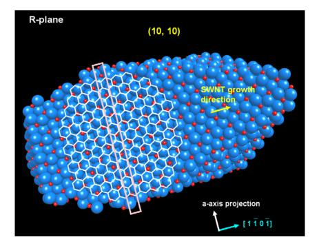
**Figure S-5.** Atomic model of *r*-plane sapphire surface overlapped with a developed (10, 10) SWNT structure. Red and blue show Al and O atoms, respectively. Although (10, 10) nanotube is metallic, we use it as a model nanotube here because of its simple structure.
