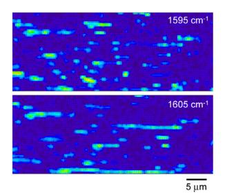
**Figure S-3.** Raman mapping images of the SWNTs grown over randomly deposited Fe-Mo catalyst, measured after the heat treatment at 1000 °C. The nanotubes were relatively short and showed wide G-band frequencies randomly distributed. The scan intervals were 0.5  $\mu$ m for both *x* and *y* directions.
