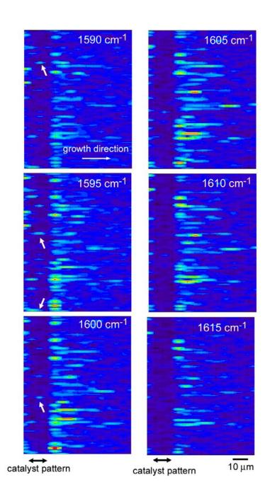
**Figure S-2.** Raman G-band mapping images of the SWNTs heat treated at 1000 °C. Inside the catalyst pattern, no significant shift in the G-band was observed (indicated by arrows). The excitation wavelength was 514.5 nm. The scan intervals were 5 and 1  $\mu$ m for *x* and *y* directions, respectively.
