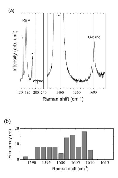
**Figure S-1.** (a) Raman spectrum of the SWNT/sapphire sample heat treated at 1000 °C. The excitation wavelength was 633 nm, and semiconducting nanotubes were detected. The sample is same with that shown in Fig. 3c. (b) Distribution of G-band frequency measured with an excitation wavelength of 633 nm. Total number of counted nanotubes is 50.
