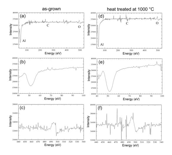
**Figure S-4.** Auger spectra of as-grown SWNTs (a-c) and those after the heat treatment at 1000 °C (d-f). (a, d) full range, (b, e) Al, (c, f) O. It is seen that relative intensity of [Al]/[O] increased after the heat treatment.
