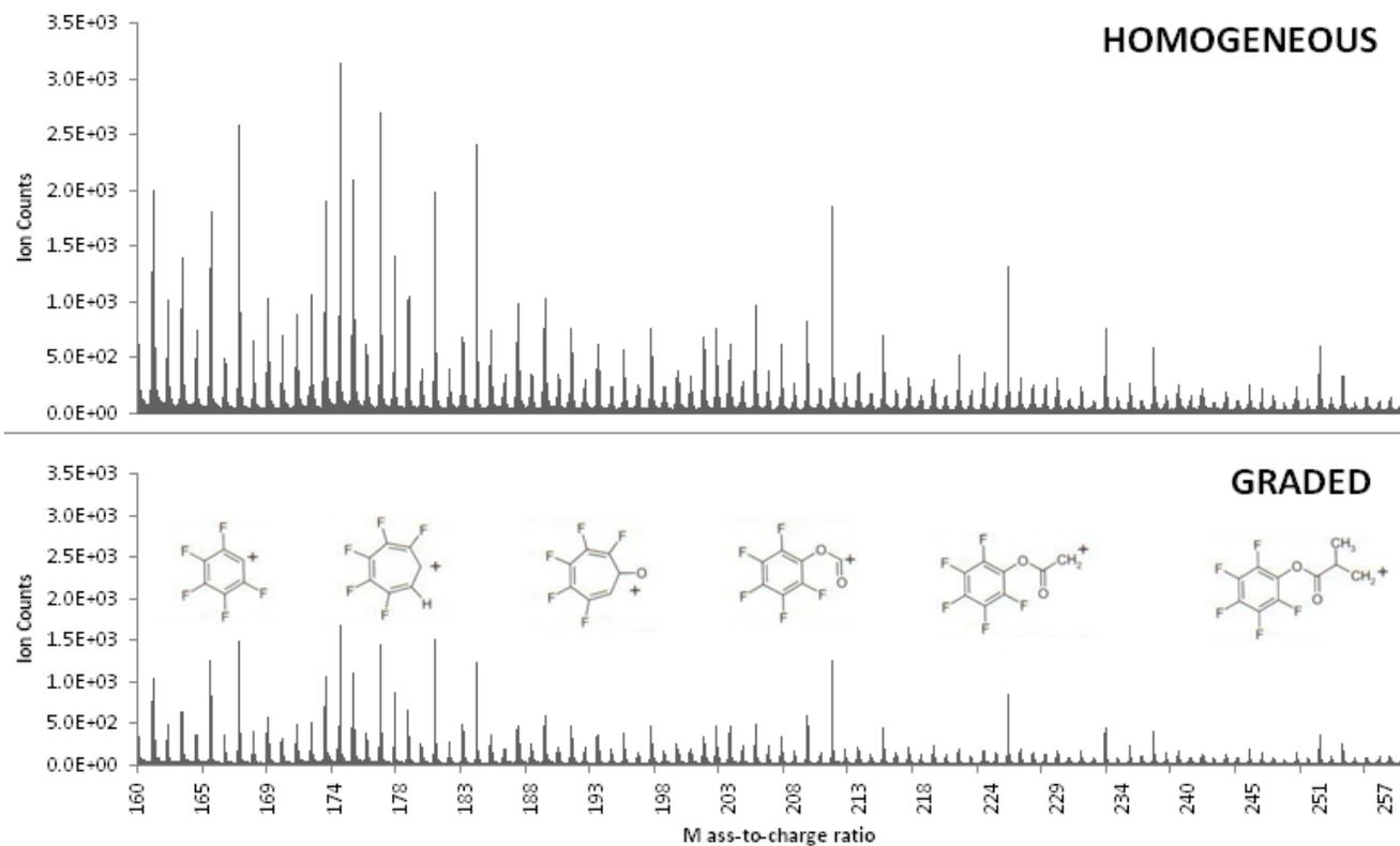
ToF-SIMS spectra of the homogeneous and graded copolymers. Characteristic peaks of the PFM comonomer are highlighted by the accompanying ionic structures.
