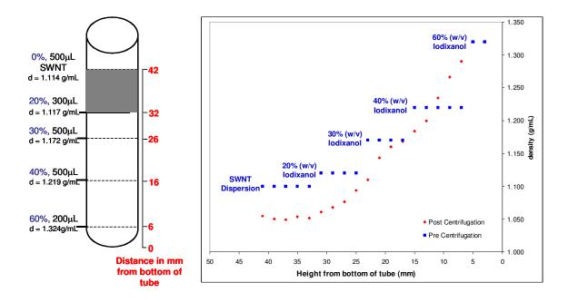
**Figure S2.** Density (g/mL) *vs* height above bottom of centrifuge tube (in mm) before (blue squares) and after (red diamonds) centrifugation.
