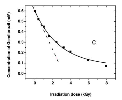
**Figure S1.** Measured loss of clofibric acid (a), bezafibrate (b) and gemfibrozil (c) in aerated aqueous solution using <sup>137</sup>Cs  $\gamma$ -irradiation. Curves correspond to fitted exponential loss, while dashed straight lines are the estimated initial slopes with values of m = -2.95 x 10<sup>-4</sup> M kGy<sup>-1</sup>, -4.29 x 10<sup>-4</sup> M kGy<sup>-1</sup>, -1.87 x 10<sup>-4</sup> M kGy<sup>-1</sup> for clofibric acid, bezafibrate and gemfibrozil respectively.
