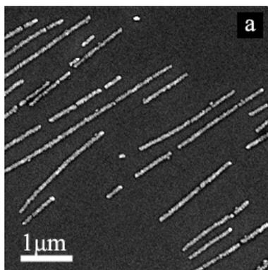
A facile and effective PDMS-transfer method is developed to fabricate highly dense and well-aligned CdS nanowires. CdS nanowires are first selectively deposited and confined on DNA template aligned on PDMS sheet, and then are transferred to the silica substrate with low occurrence of parasitic CdS nanoparticles. The width and length of nanowires can be controlled by adjusting incubation time.
