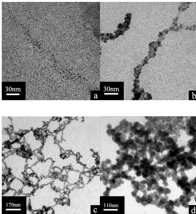
Figure S3. TEM images of CdS nanowires synthesized by solution-suspended DNA method with different molar ratios of  $\text{Cd}^{2+}$  to DNA base pairs. (a) 10:1 (b) 50:1 (c) 100:1 (d) 200:1
