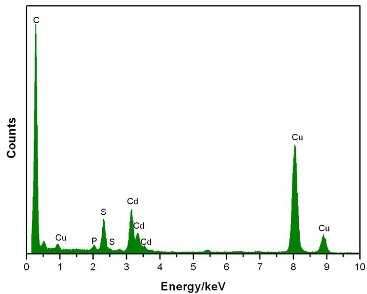
Figure S4. Energy dispersive X-ray spectrum of synthesized CdS nanowires
