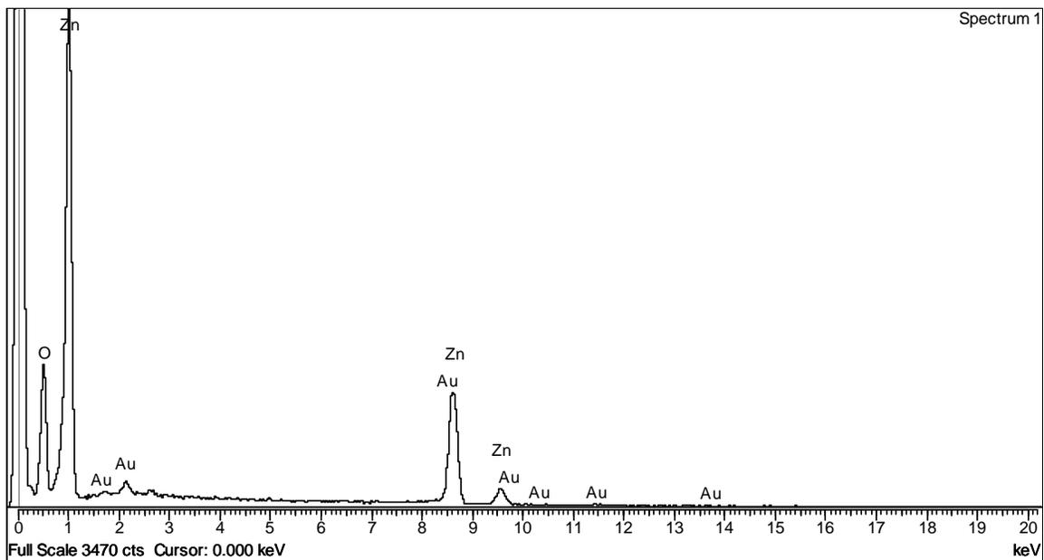
**Figure S2.** EDX analysis of an individual zinc glycolate bi-pyramidal structures. (Presence of Au is due to the gold coating that is necessary for SEM analysis of non-conductive samples)
