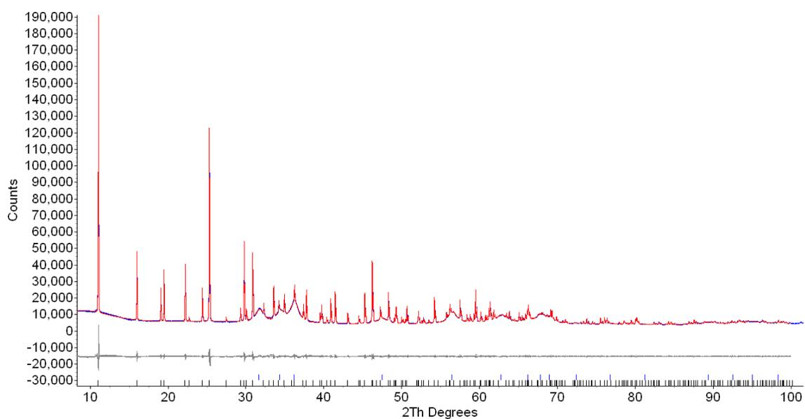
**Figure S1:** Pawley fit to the room temperature powder XRD pattern of the precursor material, showing the peaks of Zn-glycolate as the highly crystalline main phase and small amounts of poorly crystalline ZnO (wurtzite form) as a second phase.
