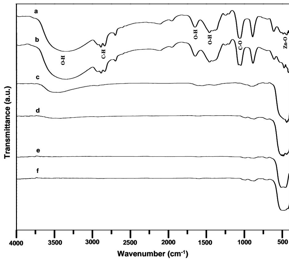
**Figure S4.** FTIR spectra that were obtained from powder samples at different temperatures. (a) Zinc glycolate, and after it has been annealed to (b) 200°C, (c) 400°C, (d) 600°C, (e) 800°C and (f) 1000°C.
