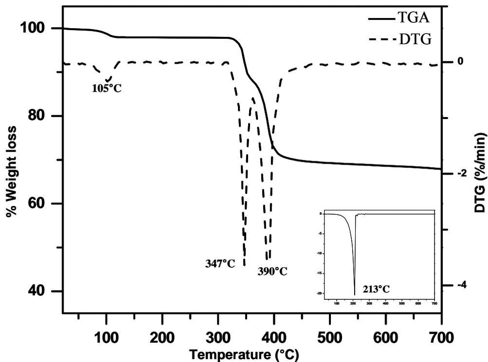
**Figure S3.** TGA curve showing the weight loss for as synthesized zinc glycolate as a function of temperature and its corresponding derivative curve (DTG). (Inset, DTG curve of pure ethylene glycol showing a peak at 213 °C)
