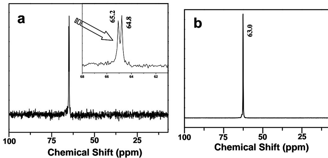
**Figure S5.** (a) Solid state CP/MAS  $^{13}\text{C}$ -NMR spectrum of zinc glycolate (inset, enlarged view revealing two distinct peaks) and (b) solution spectrum of pure ethylene glycol
