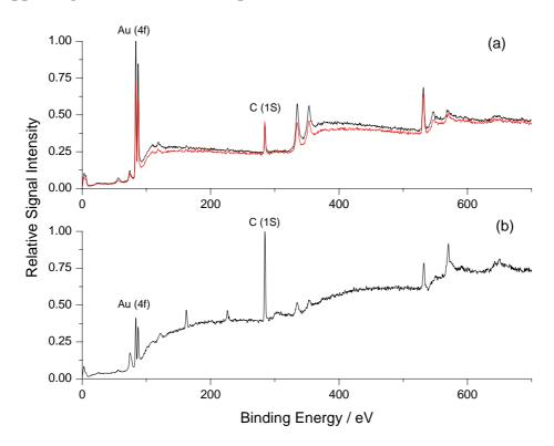
XPS spectra of  $C_6H_{13}$ -SAMs, as prepared freshly out of solution ((a) red line); in the vacuum chamber at the base pressure for 2.5 hours ((a) black line); and exposed to  $NO_2$  in reaction chamber for  $\sim 1$  hr ((b) black line).
