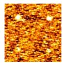
AFM topography image of sub-100 nm features produced by tips inked with one drop of 0.5 mM MHA-ethanol solution. The diameters of top and bottom row features are 90 and 75 nm, respectively.
