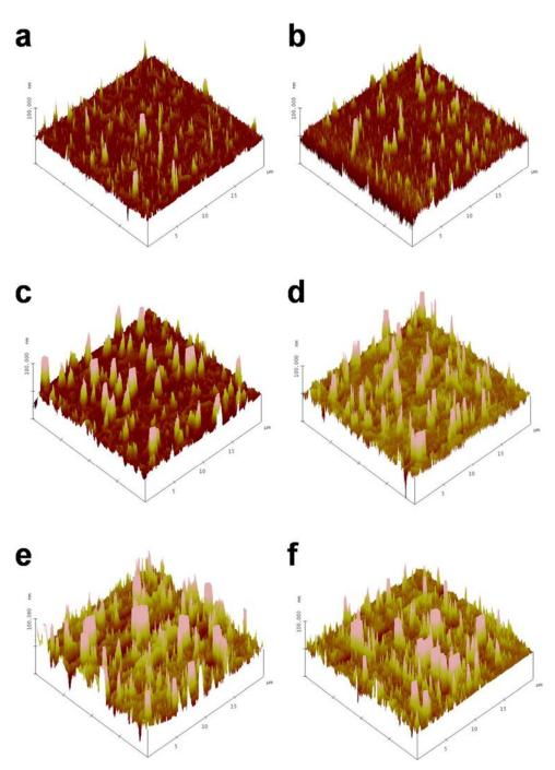
Representative tapping mode AFM images for increasing numbers of 10 mM MHA-ethanol drops on flat (RMS roughness <1.3 nm) Si<sub>x</sub>N<sub>y</sub> substrates. (a) 1 drop. (b) 2 drops. (c) 3 drops. (d) 4 drops. (e) 5 drops. (f) 6 drops. Scan area is 20  $\mu$ m × 20  $\mu$ m. Scan frequency was 1.0 Hz with 512 samples per line.
