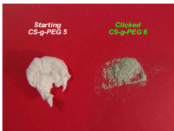
Figure S3. Picture of starting CS-g-PEG-N 3 5 (left) and clicked CS-g-PEG 6 after CuAAC (right).
