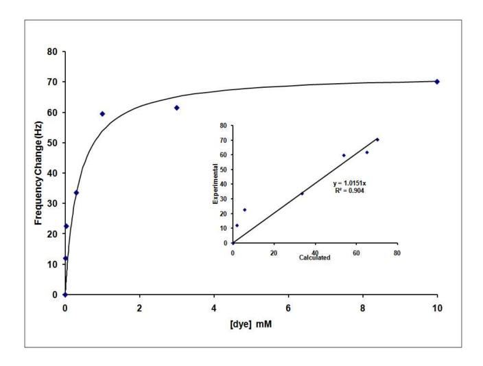
**Figure S1:** Control QCM dissociation constant experiment on a **PDDA/PSS/CT** film. The line represents the fit to a single  $K_d$  model. Inset: Values calculated using the single  $K_d$  model vs. the experimental data.
