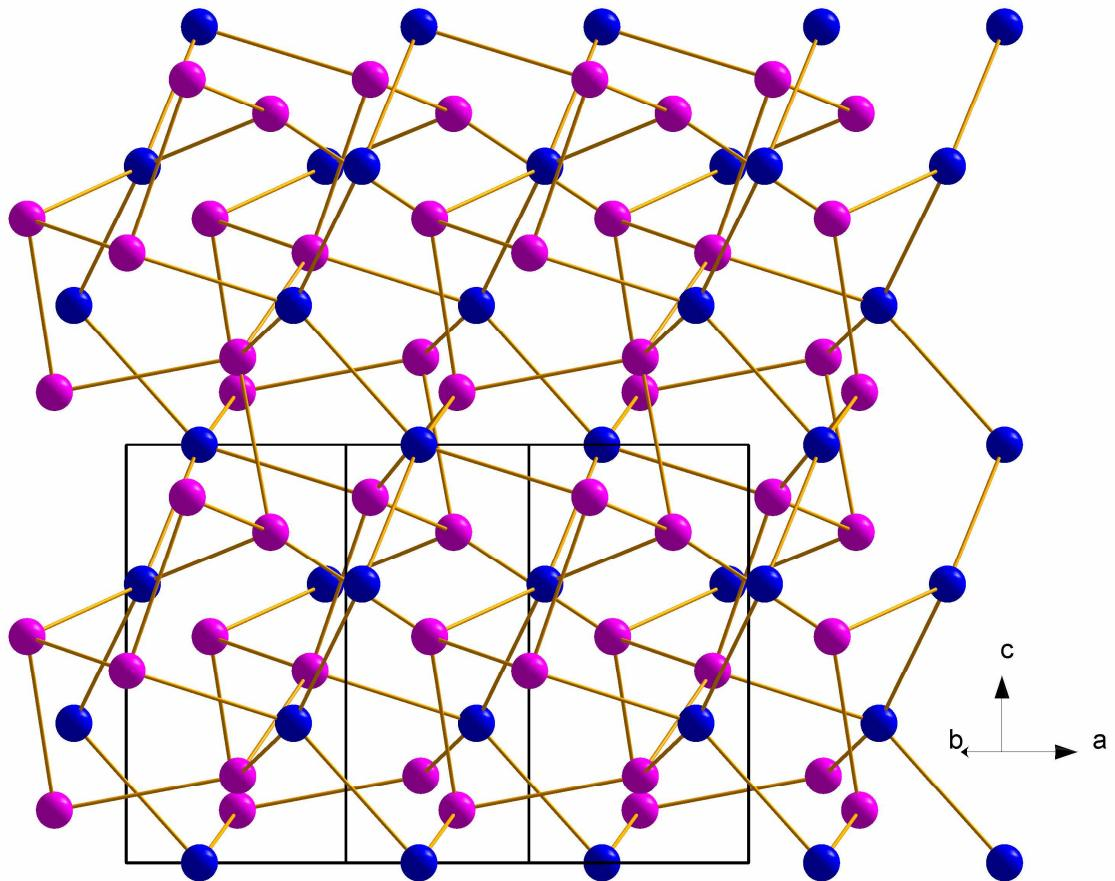
**Figure S2.** A novel tetrahedral framework topology in  $\text{Mn}(\text{BH}_4)_2$ . Four-connected Mn nodes are shown. Mn...Mn distances range from 4.71 to 4.86 Å.
