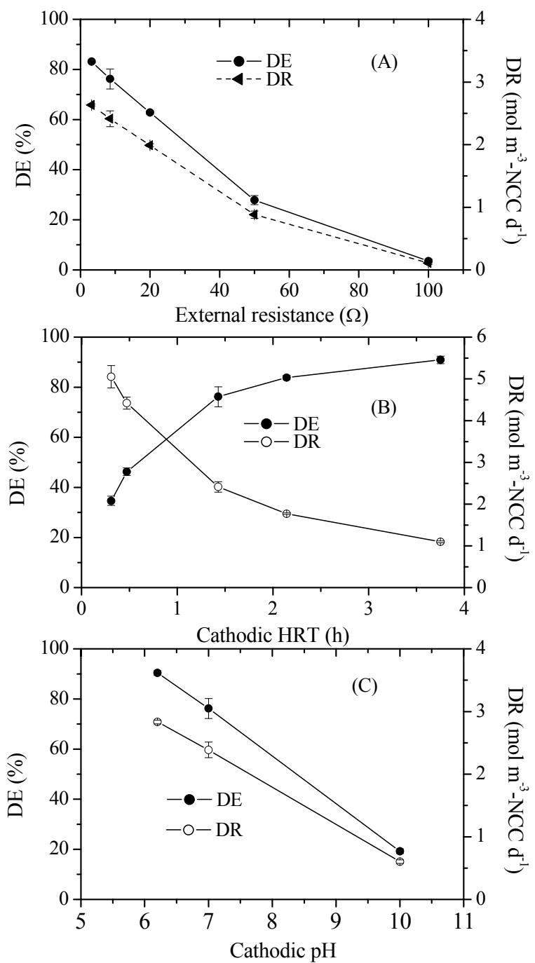
**FIGURE S1.** Effect of (A) external resistance, (B) cathodic HRT, and (C) cathodic pH on AO7 decolorization efficiency (DE) and rate (DR) in BES (A: influent AO7 0.19 mM, HRT 1.44 h, pH 7.0; B: influent AO7 0.19 mM, external resistance 8.5  $\Omega$ , pH 7.0; C: influent AO7 0.19 mM, external resistance 8.5  $\Omega$ , HRT 1.44 h).
