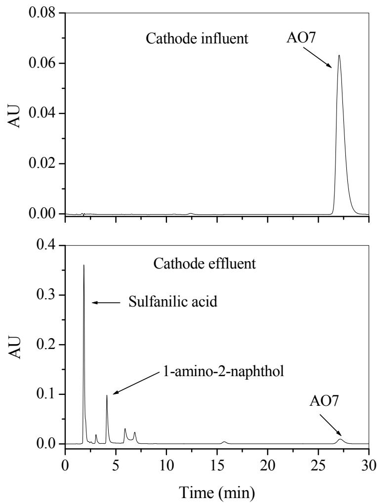
**FIGURE S3.** HPLC chromatogram of influent and effluent samples of the cathode in BESSs (AO7 concentration 0.19 mM, external resistance 8.5 Ω, HRT 1.44 h, pH).
