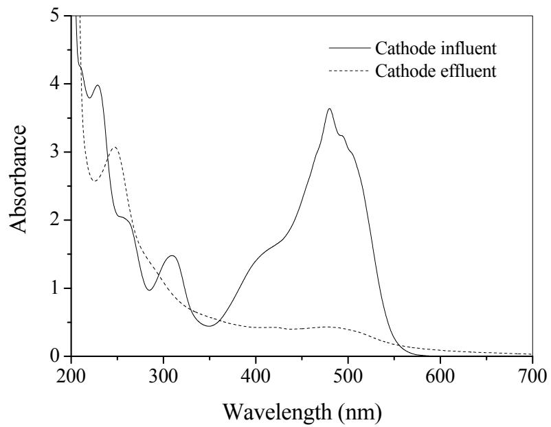
**FIGURE S2.** Evolution of UV-vis spectra for AO7 decolorization (AO7 concentration 0.19 mM, external resistance 8.5  $\Omega$ , HRT 1.44 h, pH 7.0).
