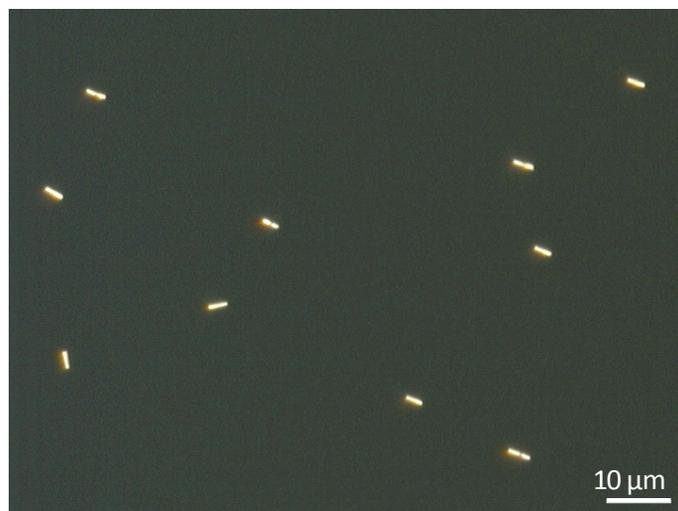
Figure S1: Optical image of the AuRu rods spin-coated onto a clean glass slide.
