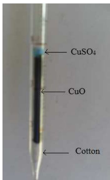
Figure S7. Tubes for testing the relative wettability of CuO colloids.
