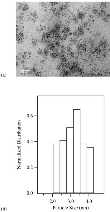
Figure S-3. (a) TEM image of PVP-capped platinum nanoparticles synthesized by reduction in the presence of methanol and (b) histogram of the particle size distribution.
