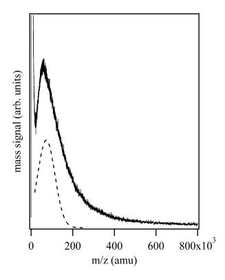
**Figure S-6.** MALDI-TOF mass spectrum of 1.85-nm PVP-capped platinum nanoparticles obtained after 200 shots from a 337-nm N<sub>2</sub> laser on sample spots from a solution of 1:10 v/v platinum nanoparticle colloid to CHCA matrix solution. The dashed line corresponds to the Gaussian curve fit for singly-charged (m/z = 73,000 amu) particles.
