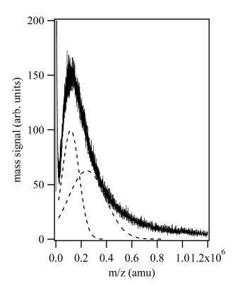
**Figure S-10.** MALDI-TOF mass spectrum of 3.69-nm PVP-capped platinum nanoparticles obtained after 200 shots from a 337-nm N<sub>2</sub> laser on sample spots from a solution of 1:10 v/v platinum nanoparticle colloid to CHCA matrix solution. The dashed lines correspond to Gaussian curve fits for triply-charged (m/z = 117,000 amu) and doubly-charged (m/z = 245,000 amu) particles.
