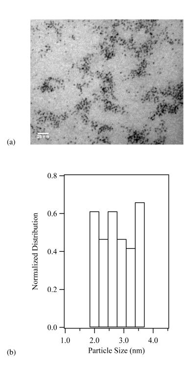
**Figure S-2.** (a) TEM image of PVP-capped platinum nanoparticles synthesized by reduction in the presence of ethanol and (b) histogram of the particle size distribution.
