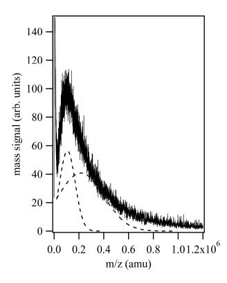
**Figure S-9.** MALDI-TOF mass spectrum of 2.94-nm PVP-capped platinum nanoparticles obtained after 200 shots from a 337-nm N<sub>2</sub> laser on sample spots from a solution of 1:10 v/v platinum nanoparticle colloid to CHCA matrix solution. The dashed lines correspond to Gaussian curve fits for doubly-charged (m/z = 107,000 amu) and singly-charged (m/z = 216,000 amu) particles.
