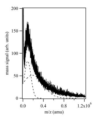
**Figure S-8.** MALDI-TOF mass spectrum of 2.60-nm PVP-capped platinum nanoparticles obtained after 200 shots from a 337-nm N<sub>2</sub> laser on sample spots from a solution of 1:10 v/v platinum nanoparticle colloid to CHCA matrix solution. The dashed lines correspond to Gaussian curve fits for doubly-charged (m/z = 93,600 amu) and singly-charged (m/z = 189,000 amu) particles.
