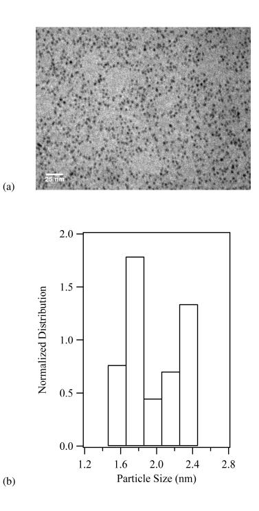
**Figure S-1.** (a) TEM image of PVP-capped platinum nanoparticles synthesized by reduction in the presence of ethylene glycol and (b) histogram of the particle size distribution.
