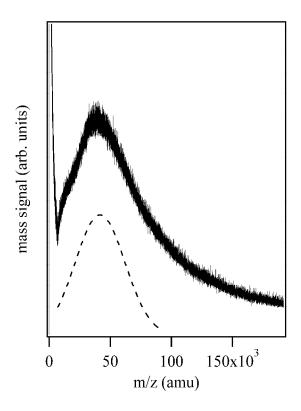
**Figure S-7.** MALDI-TOF mass spectrum of 1.85 nm uncapped platinum nanoparticles obtained after 200 shots from a 337-nm N<sub>2</sub> laser on sample spots from a solution of 1:10 v/v platinum nanoparticle colloid to CHCA matrix solution. The dashed line corresponds to the Gaussian curve fit for singly-charged (m/z = 42,000 amu) particles.
