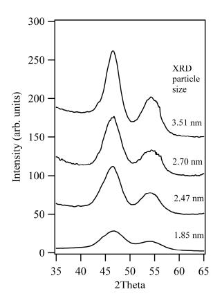
Figure S-5. XRD patterns obtained for PVP-capped platinum nanoparticles. Patterns are vertically offset for clarity.
