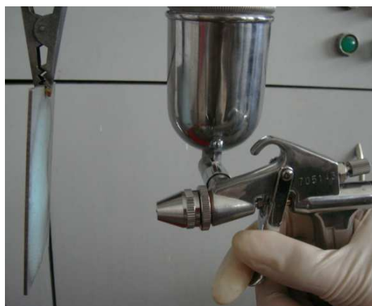
Fig.S1 Demonstration of the simple operation of spaying process for the formation of superhydrophobic coating
