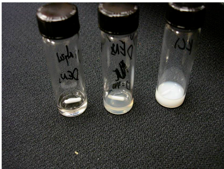
Figure S3. The results of the addition of \text{AgNO}_3 to solutions containing dialyzed DENs (left), undialyzed DENs (center), and the KCl control (right) are shown. The calculated concentration of \text{Cl}^- in undialyzed 2.0 \mu\text{M} \text{G6-OH(Pd}_{147}) DENs, introduced as \text{K}_2\text{PdCl}_4 in the starting material, is 1.18 \text{ mM} . The KCl control contained 1.18 \text{ mM} of KCl in water. A ten-fold excess of \text{Ag}^+ , with respect to this concentration of \text{Cl}^- , was added in the form of \text{AgNO}_3 to each solution. The minimum detectable amount of \text{Cl}^- was determined from the solubility product of \text{AgCl} as 13.4 \mu\text{M} using the following equilibrium equation, where K_{\text{sp}} is the solubility product for solid \text{AgCl} ( 1.8 \times 10^{-10} ).
