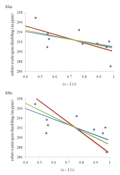
Figure S3. Nitrogen shielding in methyl nitrate as a function of solvent dielectric constant. In part a, all models have their intrinsic Coulomb radii scaled by 0.8, and in part b the radii are scaled by a factor of 1.2. Diamonds represent experimental results, the red line represents eq 11 fitted to SMD results, the blue line represents eq 11 fitted to SM8 results, and the green line represents eq 11 fitted to SM8AD results.
