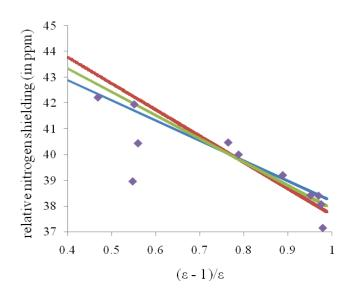
Figure S4. Nitrogen shielding in nitromethane as a function of solvent dielectric constant. In part a, all models have their intrinsic Coulomb radii scaled by 0.8, and in part b the radii are scaled by a factor of 1.2. Diamonds represent experimental results, the red, blue, and green lines represent eq 11 fitted to SMD, SM8, and SM8AD results, respectively. In part a, the blue and red lines are almost covered by the SM8AD line, and in part b the blue line is behind the green one.
