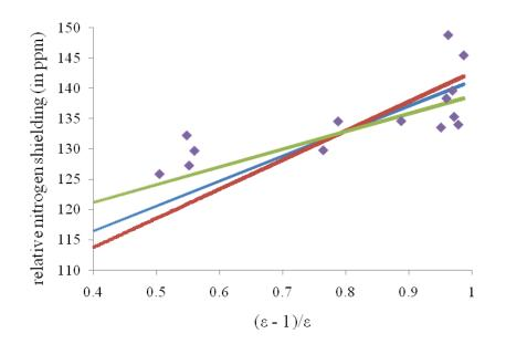
Figure S2. Nitrogen shielding in methyl isothiocyanate as a function of solvent dielectric constant. In part a, all models have their intrinsic Coulomb radii scaled by 0.8, and in part b the radii are scaled by a factor of 1.2. Diamonds represent experimental results, the red line represents eq 11 fitted to SMD results, the blue line represents eq 11 fitted to SM8 results, and the green line represents eq 11 fitted to SM8AD results.
