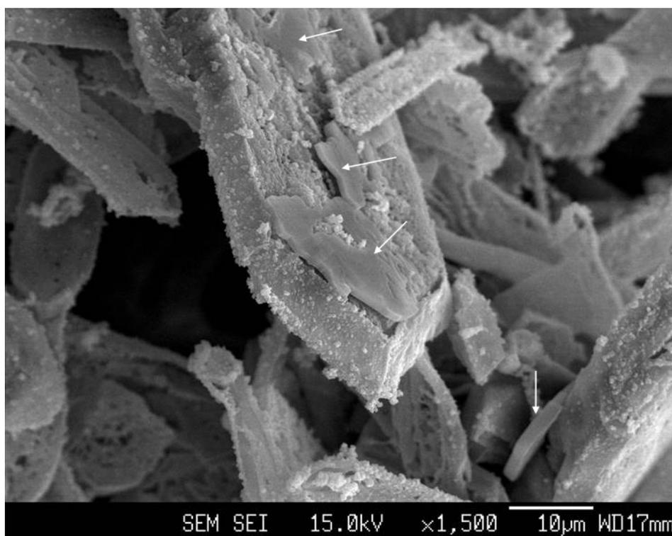
**Figure S5. SEM image of the KSBA crystals at polymerization  $t = 60$  min.** White arrows indicate the fragments of the KSBA crystals by continuous dissolution and mechanical stirring. Therefore, the PPy structure patterned after the pre-existing KSBA crystal is easily separated from the KSBA crystal.
