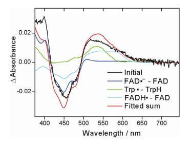
**Figure S5**. The initial spectrum was reproduced in a fitting procedure by including FAD neutral and anion radicals and the tryptophan neutral radical. Strong deviations of the fitted sum from the measured spectrum illustrate that the flavin neutral radical cannot account for the absorption at 550-600 nm.
