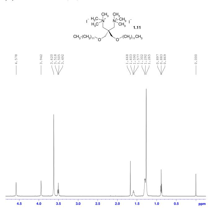
Expansion of part of the 500.1 MHz  $^{1}$ H NMR spectrum of 2,2-bis(dodecyloxymethyl)-N,N,N,N,N-hexamethyl-1,3-propanediammonium diiodide (**1.11**) in CDCl<sub>3</sub>
