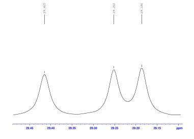
$500.1\,\text{MHz}$   $^1\text{H}$  NMR spectrum of 1,3-bis(1-azacyclopentyl)-2,2-bis(decyloxymethyl)propane dihydrochloride (1.18) in CDCl $_3$
