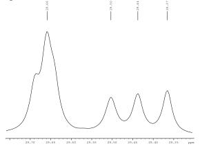
500.1 MHz  $^1$ H NMR spectrum of N,N,N',N'-tetramethyl-2,2-bis(tetradecyloxymethyl)-1,3-propanediaminium dichloride (**1.8**) in chloroform-d
