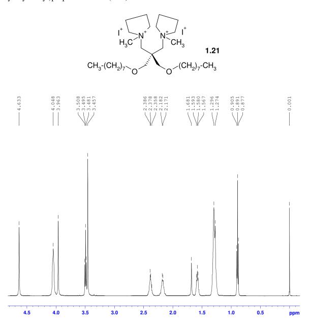
Expansion of part of the 500.1 MHz  $^1$ H NMR spectrum of 1,3-bis(1-methyl-1-azoniacyclopentyl)-2,2 bis(octyloxymethyl) propane diiodide (**1.21**) in CDCl<sub>3</sub>
