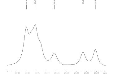
500.1 MHz  $^1$ H NMR spectrum of 1,3-bis(1-azacyclopentyl)-2,2-bis(octyloxymethyl)propane dihydrochloride (1.17) in chloroform-d
