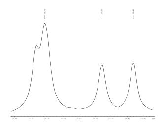
500.1 MHz  $^1$ H NMR spectrum of 2,2-bis(dodecyloxymethyl)-N,N,N,N,N,N-hexamethyl-1,3-propanediammonium diiodide (**1.11**) in chloroform-d
