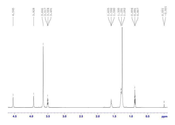
Expansion of part of the 500.1 MHz  $^{1}$ H NMR spectrum of N,N,N,N',N',N'-hexamethyl-2,2-bis(tetradecyloxymethyl)-1,3-propanediammonium diiodide (**1.12**) in chloroform-d
