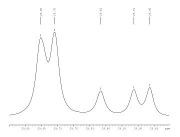
500.1 MHz  $^1$ H NMR spectrum of 1,3-bis(1-methyl-1-azoniacyclopentyl)-2,2 bis(octyloxymethyl)propane diiodide (**1.21**) in chloroform-d
