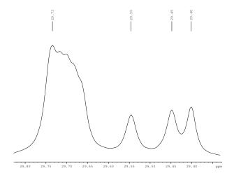
500.1 MHz  $^1$ H NMR spectrum of N,N,N,N',N'-hexamethyl-2,2-bis(octyloxymethyl)-1,3-propanediammonium diiodide (**1.9**) in chloroform-d
