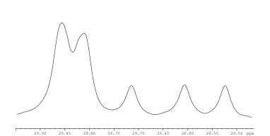
500.1 MHz  $^1$ H NMR spectrum of N,N,N',N'-tetramethyl-2,2-bis(octyloxymethyl)-1,3-propanediaminium dichloride (**1.5**) in chloroform-d
