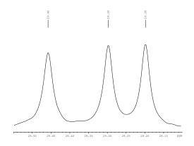
500.1 MHz  $^1$ H NMR spectrum of N,N,N',N'-tetramethyl-2,2-bis(decyloxymethyl)-1,3-propanediaminium dichloride (**1.6**) in chloroform-d
