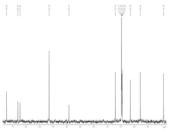
Expansion of part of the 125.7 MHz  $^{13}$ C NMR spectrum of 2,2-bis(dodecyloxymethyl)-N,N,N,N,N,N-hexamethyl-1,3-propanediammonium diiodide (**1.11**) in CDCl<sub>3</sub>
