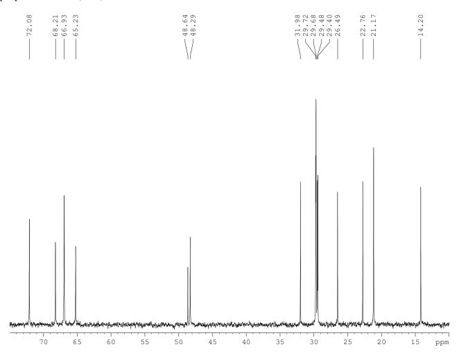
Expansion of part of the 125.7 MHz <sup>13</sup>C NMR spectrum of 2,2 bis(decyloxymethyl)-1,3-bis(1-methyl-1-azoniacyclopentyl)propane diiodide (**1.22**) in CDCl<sub>3</sub>
