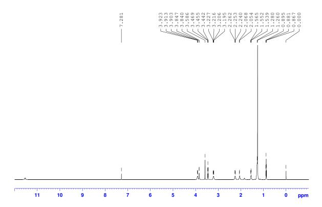
Expansion of part of the 500.1 MHz  $^1$ H NMR spectrum of 1,3-bis(1-azacyclopentyl)-2,2-bis(tetradecyloxymethyl)propane dihydrochloride (**1.20**) in CDCl<sub>3</sub>
