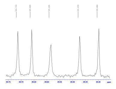
500.1 MHz  $^1$ H NMR spectrum of 1,3-bis(1-azacyclopentyl)-2,2-bis(dodecyloxymethyl)propane dihydrochloride (**1.19**) in chloroform-d
