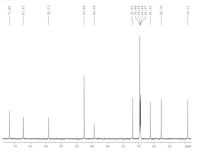
Expansion of part of the 125.7 MHz  $^{13}$ C NMR spectrum of N,N,N',N'-tetramethyl-2,2-bis(dodecyloxymethyl)-1,3-propanediaminium dichloride (1.7) in CDCl<sub>3</sub>
