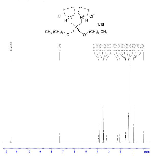
Expansion of part of the 500.1 MHz  $^1$ H NMR spectrum of 1,3-bis(1-azacyclopentyl)-2,2-bis(decyloxymethyl)propane dihydrochloride (**1.18**) in CDCl $_3$
