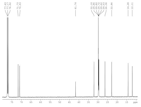
Expansion of part of the 125.7 MHz  $^{13}$ C NMR spectrum of 2,2'-bis(dodecyloxymethyl)-1,3-diiodopropane (15) in CDCl<sub>3</sub>
