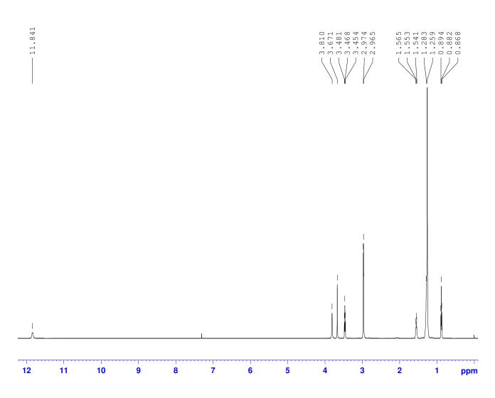
Expansion of part of the 500.1 MHz <sup>1</sup>H NMR spectrum of *N*,*N*,*N*',*N*'-tetramethyl-2,2-bis(tetradecyloxymethyl)-1,3-propanediaminium dichloride (**1.8**) in CDCl<sub>3</sub>
