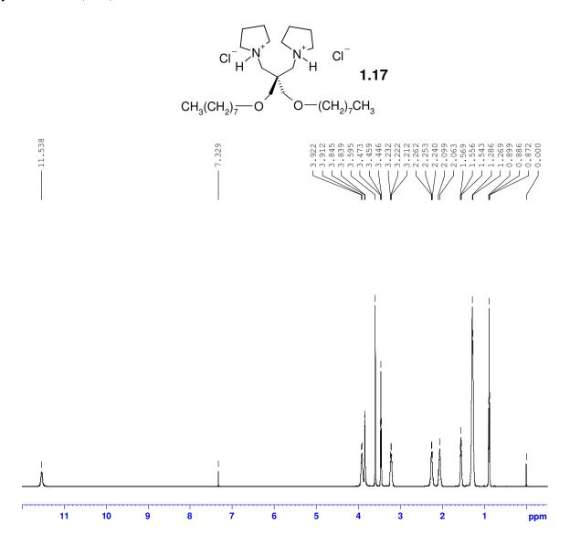
Expansion of part of the 500.1 MHz  $^1$ H NMR spectrum of 1,3-bis(1-azacyclopentyl)-2,2-bis(octyloxymethyl)propane dihydrochloride (**1.17**) in CDCl<sub>3</sub>
