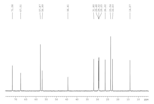
Expansion of part of the 125.7 MHz <sup>13</sup>C NMR spectrum of 1,3-bis(1-azacyclopentyl)-2,2-bis(octyloxymethyl)propane dihydrochloride (**1.17**) in CDCl<sub>3</sub>
