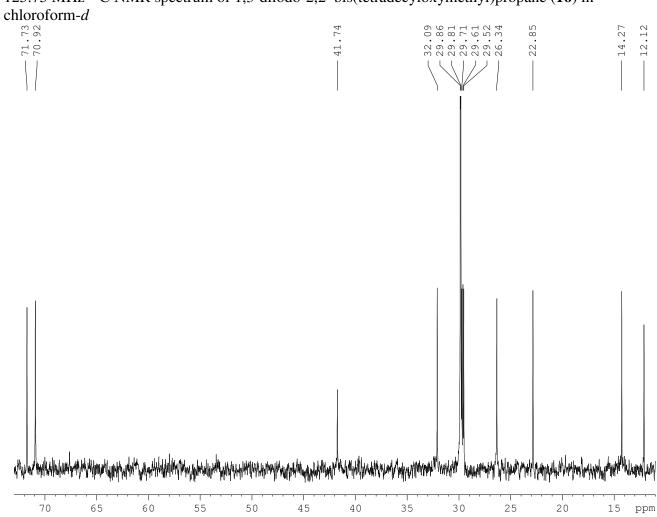
Expansion of part of the 125.7 MHz  $^{13}$ C NMR spectrum of 1,3-diiodo-2,2'bis(tetradecyloxymethyl)propane (16) in CDCl<sub>3</sub>
