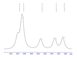
500.1 MHz  $^1$ H NMR spectrum of 1,3-bis(1-azacyclopentyl)-2,2-bis(tetradecyloxymethyl)propane dihydrochloride (**1.20**) in chloroform-d
