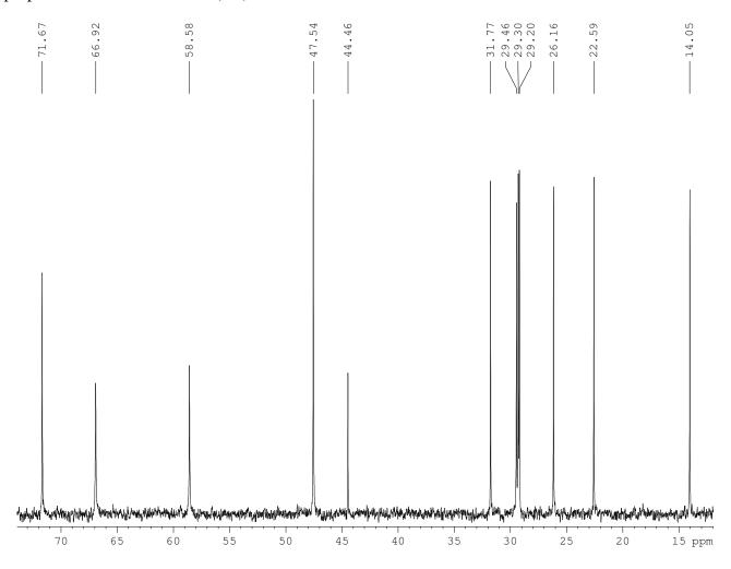
Expansion of part of the 125.7 MHz  $^{13}$ C NMR spectrum of N,N,N',N'-tetramethyl-2,2-bis(octyloxymethyl)-1,3-propanediaminium dichloride (1.5) in CDCl<sub>3</sub>
