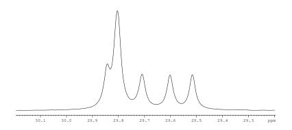
500.1 MHz  $^1\mathrm{H}$  NMR spectrum of 1,3-diiodo-2,2'-bis(tetradecyloxymethyl)propane (16) in chloroform- d
