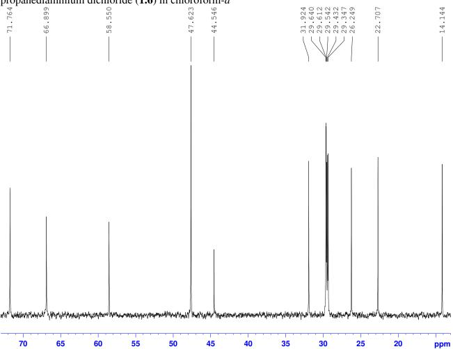
Expansion of part of the 125.7 MHz  $^{13}$ C NMR spectrum of N,N,N',N'-tetramethyl-2,2-bis(decyloxymethyl)-1,3-propanediaminium dichloride (**1.6**) in CDCl<sub>3</sub>
