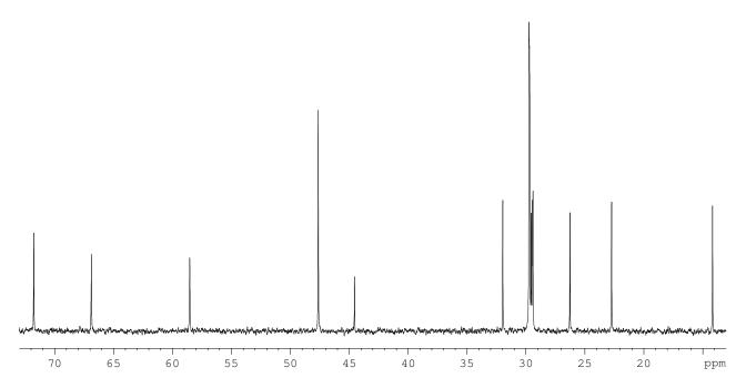
Expansion of part of the 125.7 MHz <sup>13</sup>C NMR spectrum of *N,N,N',N'*-tetramethyl-2,2-bis(tetradecyloxymethyl)-1,3-propanediaminium dichloride (**1.8**) in CDCl<sub>3</sub>
