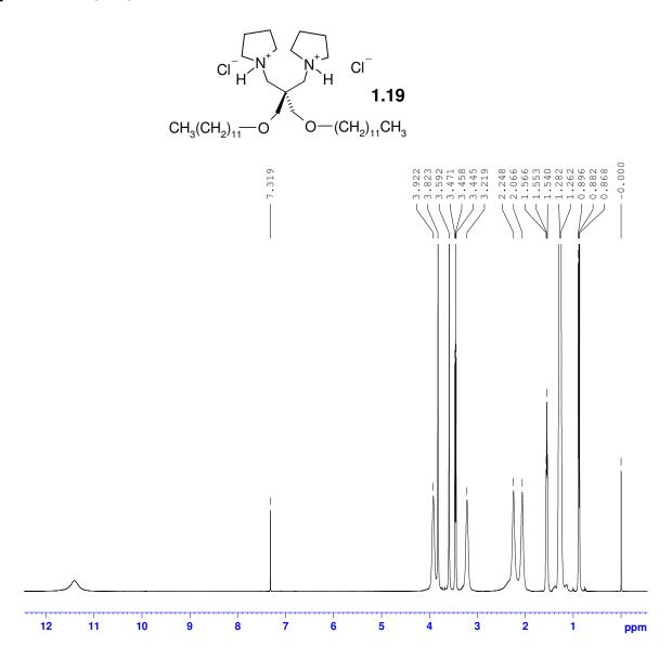
Expansion of part of the 500.1 MHz  $^1$ H NMR spectrum of 1,3-bis(1-azacyclopentyl)-2,2-bis(dodecyloxymethyl)propane dihydrochloride (**1.19**) in CDCl<sub>3</sub>
