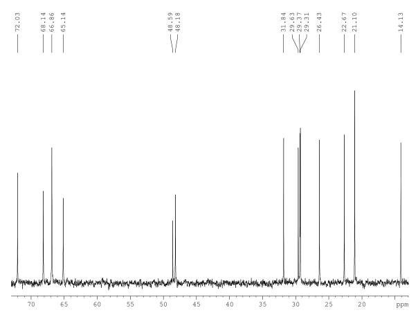
Expansion of part of the 125.7 MHz <sup>13</sup>C NMR spectrum of 1,3-bis(1-methyl-1-azoniacyclopentyl)-2,2 bis(octyloxymethyl)propane diiodide (**1.21**) in CDCl<sub>3</sub>
