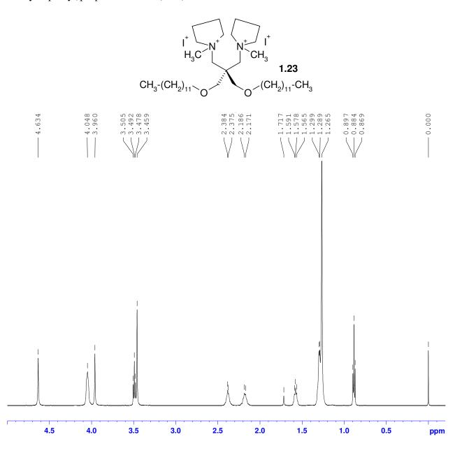
Expansion of part of the 500.1 MHz  $^1$ H NMR spectrum of 2,2-bis(dodecyloxymethyl)-1,3-bis(1-methyl-1-azoniacyclopentyl)propane diiodide (**1.23**) in chloroform-d
