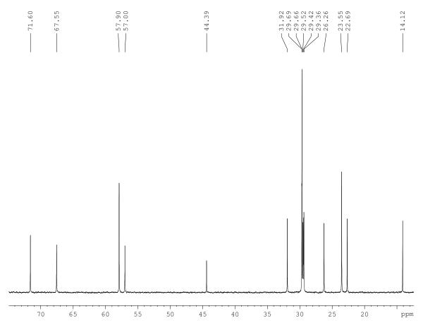
Expansion of part of the 125.7 MHz <sup>13</sup>C NMR spectrum of 1,3-bis(1-azacyclopentyl)-2,2-bis(dodecyloxymethyl)propane dihydrochloride (**1.19**) in CDCl<sub>3</sub>
