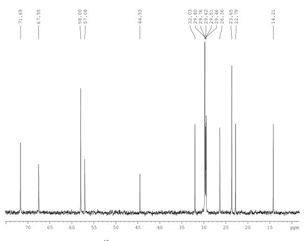
Expansion of part of the 125.7 MHz  $^{13}$ C NMR spectrum of 1,3-bis(1-azacyclopentyl)-2,2-bis(tetradecyloxymethyl)propane dihydrochloride (**1.20**) in CDCl<sub>3</sub>
