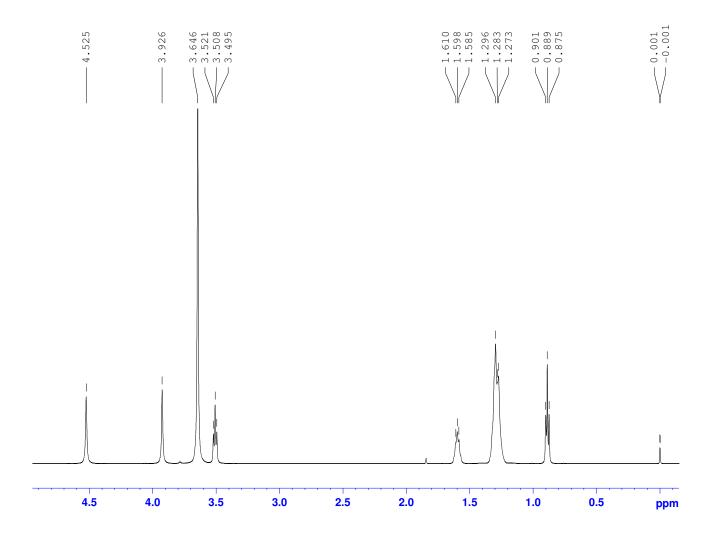
Expansion of part of the 500.1 MHz  $^{1}$ H NMR spectrum of N,N,N,N',N',N'-hexamethyl-2,2-bis(octyloxymethyl)-1,3-propanediammonium diiodide (**1.9**) in chloroform-d
