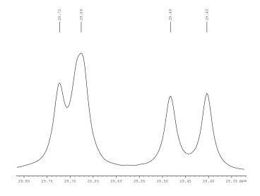
500.1 MHz  $^1$ H NMR spectrum of 2,2-bis(dodecyloxymethyl)-1,3-bis(1-methyl-1-azoniacyclopentyl)propane diiodide (**1.23**) in chloroform-d
