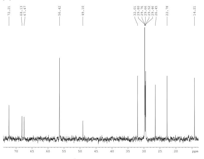
Expansion of part of the 125.7 MHz  $^{13}$ C NMR spectrum of N,N,N,N',N',N'-hexamethyl-2,2-bis(tertradecyloxymethyl)-1,3-propanediammonium diiodide (**1.12**) in chloroform-d
