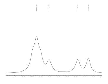
500.1 MHz  $^1$ H NMR spectrum of N,N,N,N',N',N'-hexamethyl-2,2-bis(tetradecyloxymethyl)-1,3-propanediammonium diiodide (**1.12**) in chloroform-d
