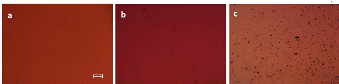
Figure S1: Dispersion of AuNPs in 50:50 mixture of 6OCB/CB15 BP: a- 2 wt.% of AuNPs, b- 25 wt.% of AuNPs, and c- 50 wt.% of AuNPs. The images show that particles are fully dispersed in BP mixtures even at higher concentrations. (Scale bar 100 \mu\text{m} ).
