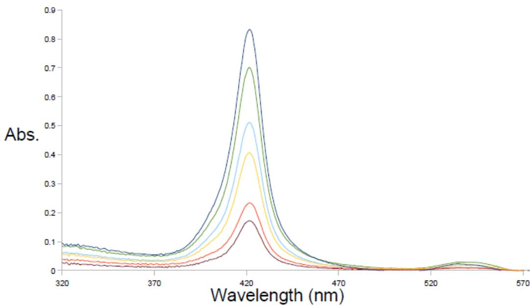
**Figure S14.** UV-Vis data for complex **4** recorded in  $\text{CH}_2\text{Cl}_2$ . This figure shows that the Soret position is independent of concentration in solution. As the concentration of complex **4** is increased (moving from the purple to the dark blue line) no change in Soret position is observed. This result implies that no intermolecular binding of the IM tether is occurring (see text for explanation).
