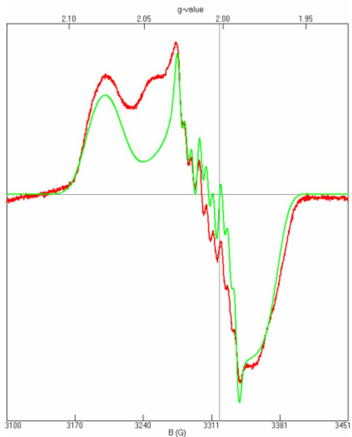
**Figure S12.** EPR spectrum of  $[\text{Fe}(\text{To-F}_2\text{PP-BzIM})(\text{NO})]$  (**4**) in frozen DMSO at 77 K (red) and fit of the spectrum using the program SpinCount (green).<sup>1</sup> Fit parameters:  $g_x = 2.077$ ,  $g_y = 2.009$ ,  $g_z = 1.978$ ;  $^{14}\text{N}$  hyperfine:  $^{^{\text{NO}}}\text{A}_x = 37$  MHz,  $^{^{\text{NO}}}\text{A}_y = 62$  MHz,  $^{^{\text{NO}}}\text{A}_z = 39$  MHz;  $^{^{\text{IM}}}\text{A}_y = 19$  MHz.
