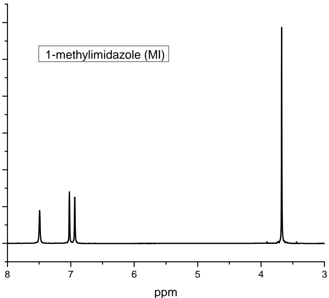
**Figure S17.**  ${}^1\text{H}$ -NMR data obtained for 1-methylimidazole (MI) in deuterated acetone. The aromatic protons are observed as singlets as in the case of our imidazole (IM) tethered porphyrins, indicating very weak couplings between the IM ring protons.
