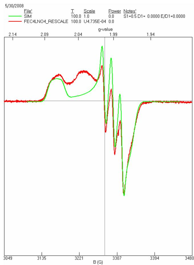
**Figure S11.** EPR spectrum of  $[\text{Fe}(\text{To}-\text{F}_2\text{PP}-\text{C}_4\text{IM})(\text{NO})]$  (**3**) recorded at 77 K in frozen toluene (red) and fit of the spectrum using the program SpinCount (green).<sup>1</sup> Fit parameters:  $g_x = 2.073$ ,  $g_y = 1.9905$ ,  $g_z = 1.971$ ;  $^{14}\text{N}$  hyperfine:  $^{NO}A_x = 39$  MHz,  $^{NO}A_y = 57$  MHz,  $^{NO}A_z = 37$  MHz;  $^{IM}A_y = 2$  MHz.
