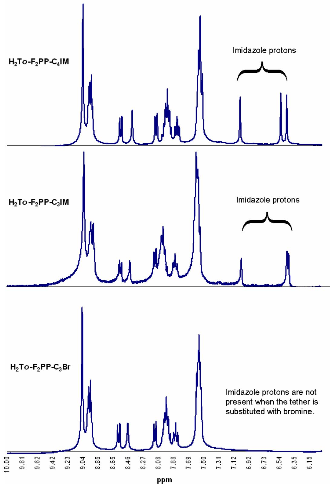
**Figure S15.** Overlay of  $^1\text{H}$ -NMR data obtained for the alkyl chain substituted ligands **L2** and **L3** as compared to  $\text{H}_2\text{To-F}_2\text{PP-C}_3\text{Br}$  where imidazole has been replaced by bromine.
