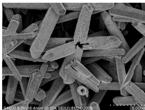
Fig. SI3 The SEM image of ZnO samples obtained without CMC at 120 °C under hydrothermal conditions
