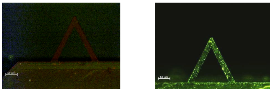
Figure 5S Fluorescence images of AFM tip a) before biotin coupling; b) after biotin coupling. Biotin(5-fluorescein) (Fluka, 53608) was used for this experiment. Coupling conditions: DCM: 2 ml; DIC: 0.5 g; biotin (5-fluorescein): 1 mg; time: 30 min. Clear contrast of fluorescence intensity before and after modification verified the successful modification of AFM tip by biotin.
