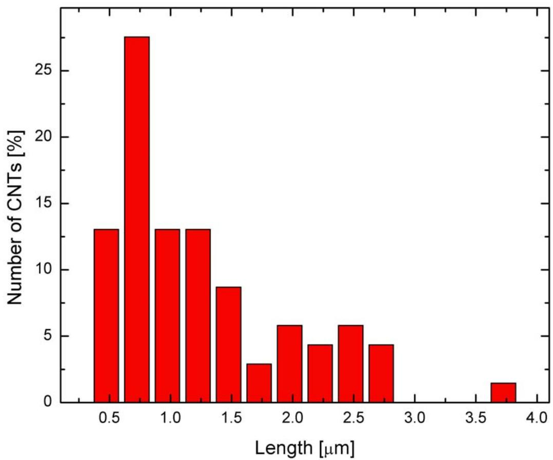
Figure S1. Carbon nanotubes length distribution determined from a large number of scanning electron micrographs.
