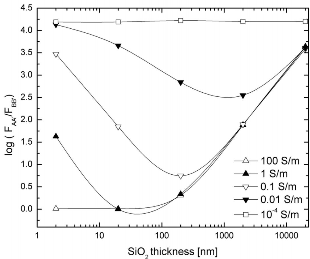
Figure S4. The attracting force on a CNT placed between the two electrodes ( $F_{AA'}$ ) and between the substrate and the active electrode ( $F_{BB'}$ ) are in competition, their relative strengths depend on the  $\text{SiO}_2$  thickness in a non-linear way
