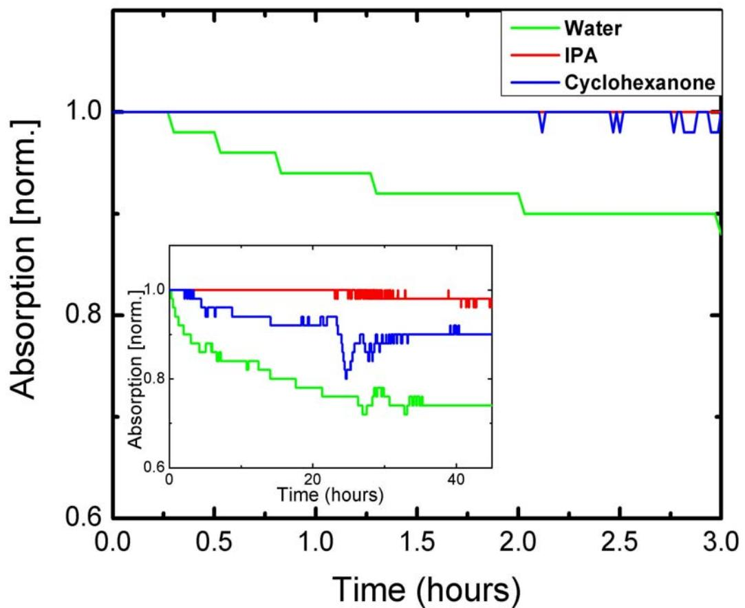
Figure S2. Normalized optical absorption (at wavelength 500 nm) measurements of CNTs dispersed into cyclohexanone, water and IPA, measured over 10 days each two minutes
