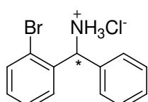
**(+)-(2-bromophenyl)(phenyl)methanaminium chloride (2b)<sup>3</sup>:**  $[\alpha]_D^{20} + 20.1$  ( $c$  1.0, MeOH), 91% ee; SFC condition for corresponding acetamide: Sepapak-4 column, MeOH with
