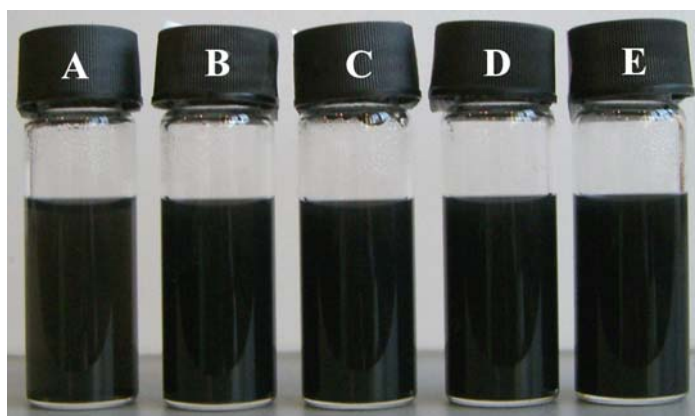
Figure S1. Dispersions of MWNTs in 3 mL of 0.1 wt % C_{12}E_6 aqueous solutions with increasing amount of added MWNTs. The weight percents of MWNTs in the preformed dispersions are 0.01 wt% (A), 0.03 wt% (B), 0.05 wt% (C), 0.06 wt% (D), 0.1 wt% (E). The images were taken more than two weeks after preparation.
