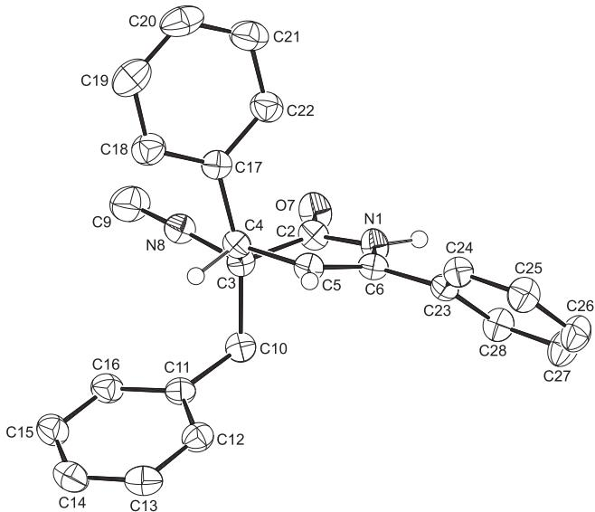
Figure S1. Displacement ellipsoid plot of **12u**, drawn at the 50% probability level. The compound was crystallized by slow diffusion of pentane into a saturated solution of **12u** in EtOAc as a racemate in the centrosymmetric space group  $P\bar{1}$ . Phenyl- and benzyl-hydrogens are omitted for clarity.
