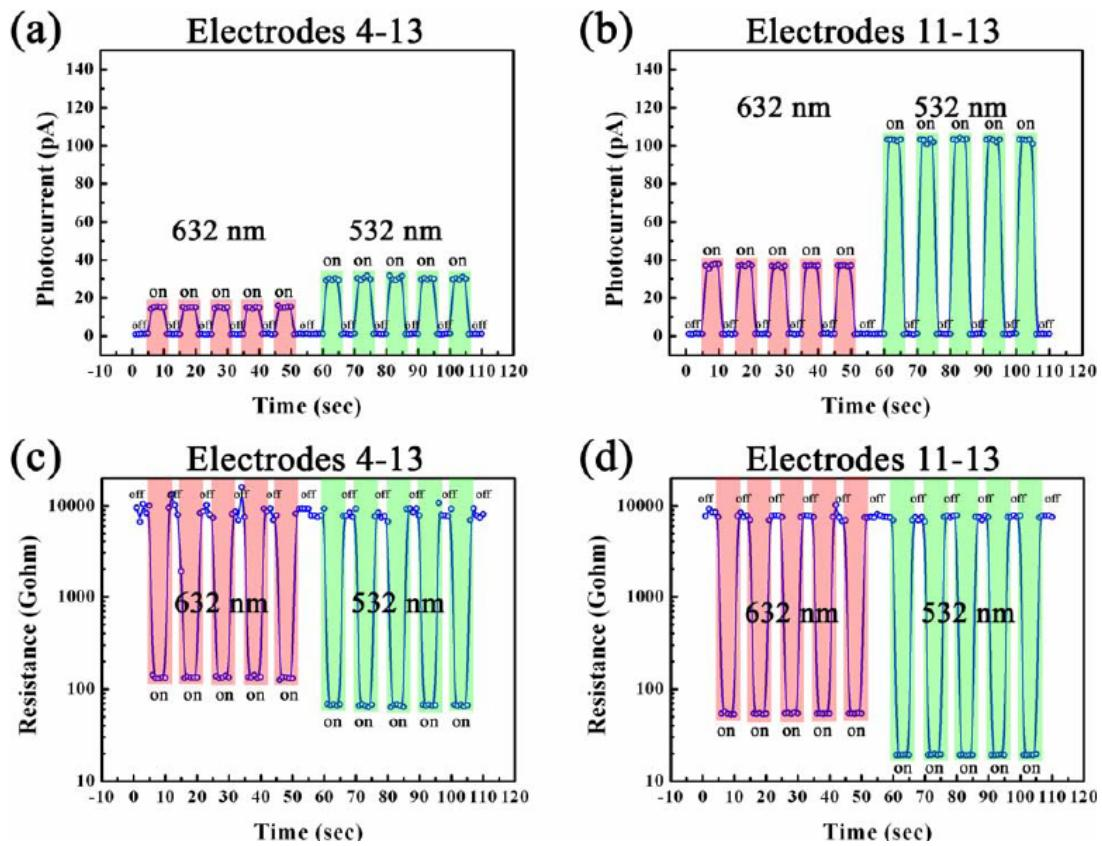
Figure S3. (a) and (b) Photo-response behaviors of illumination-on and -off cycles between No. 4-13 and No. 11-13 electrodes, respectively. (c) and (d) show the corresponding re-plotted figures of resistance vs. time.
