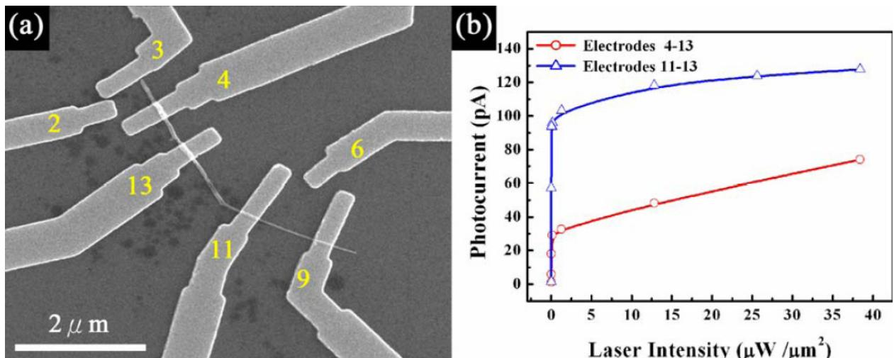
Figure S2. (a) High-magnification SEM image and (b) photo-response behaviors of a gold-in-Ga<sub>2</sub>O<sub>3</sub> peapoded nanowire with average gold diameter of 40 nm.
