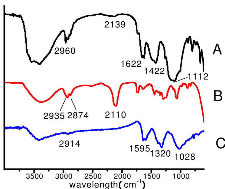
**Figure.S2** FT-IR spectra of (A) alkynyl-Ag NPs (B) 2-azidoethanol (C) triazole-Ag NPs
