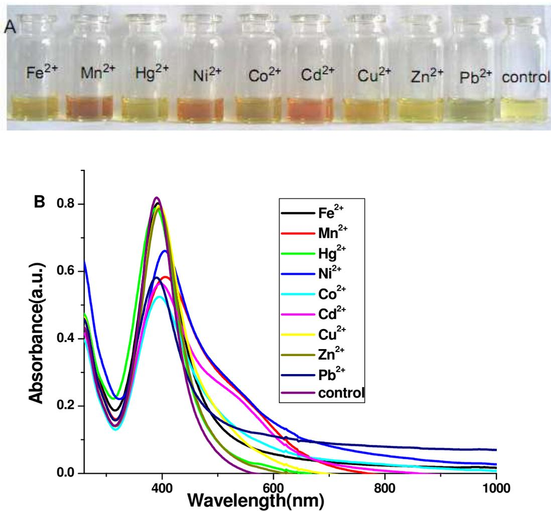
**Figure. S8** The photographic image (A) and UV-*vis* absorption spectra (B) of alkynyl-carboxyl Ag NPs solution after adding transition metal ions (10  $\mu$ M) for 5 mins. Typically, 0.5 mL of 50  $\mu$ M various transition metal ions were added into 2 mL alkynyl-carboxyl Ag NPs solutions and the combined solution mixed well for 5 mins and then tested.
