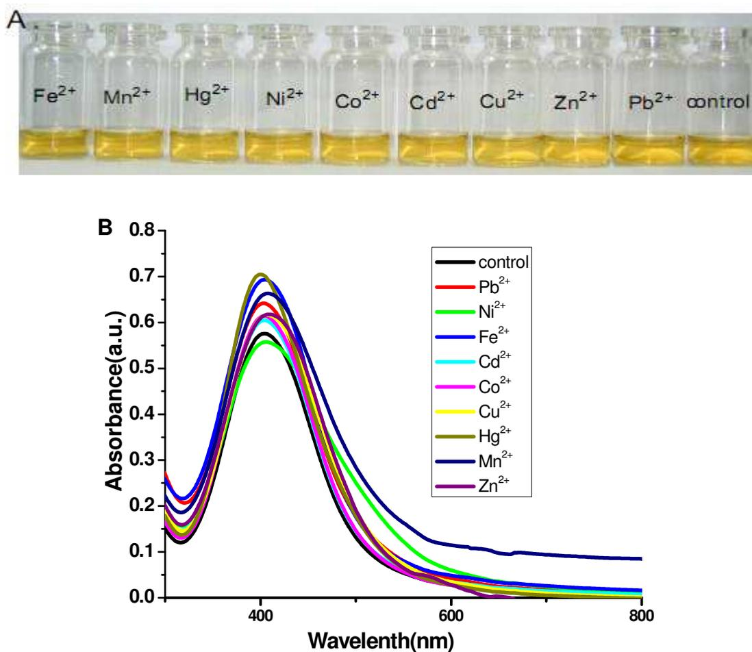
**Figure. S6** The photographic images (A) and UV-*vis* absorption spectra (B) of triazole-Ag NPs solution after adding transition metal ions (10  $\mu$ M) for 5 mins. Typically, 0.5 mL of 50  $\mu$ M various transition metal ions were added into 2 mL triazole-Ag NPs solutions and the combined solution mixed well for 5 mins and then tested.
