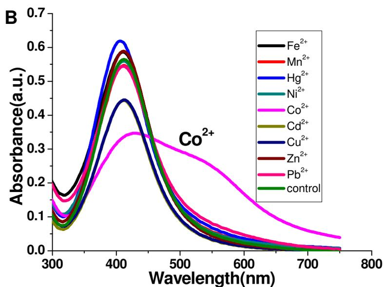
**Figure.S4** The photographic images (A) and UV-*vis* absorption spectra (B) of triazole-carboxyl Ag NPs solution after adding transition metal ions (10  $\mu\text{M}$ ) for 5 mins. Typically, 0.5 mL of 50  $\mu\text{M}$  various transition metal ions were added into 2 mL triazole-Ag NPs solutions and the combined solution mixed well for 5 mins and then tested.
