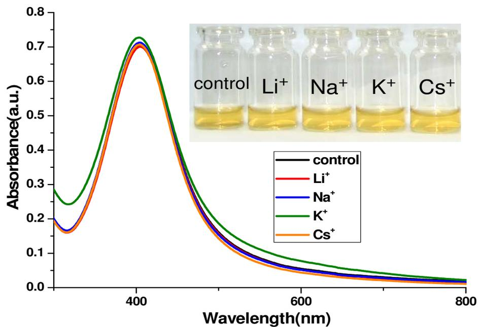
**Figure.S7** The UV-*vis* absorption spectra and photographic images (inset) of triazole-carboxyl Ag NPs solution in the presence of 10 μM different metal ions. Typically, 0.5 mL of 50 μM various transition metal ions were added into 2 mL triazole-carboxyl Ag NPs solutions and the combined solution mixed well for 5 mins and then tested.
