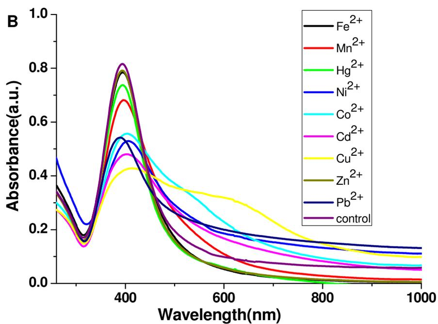
**Figure S5** The photographic image (A) and UV-*vis* absorption spectra (B) of 2-mercaptoacetic acid modified Ag NPs (carboxyl-Ag NPs) solution after adding transition metal ions ( $50 \mu\text{M}$ ) for 5 mins. Typically,  $0.5 \text{ mL}$  of  $50 \mu\text{M}$  various transition metal ions were added into  $2 \text{ mL}$  carboxyl-Ag NPs solutions and the combined solution mixed well for 5 mins and then tested.
