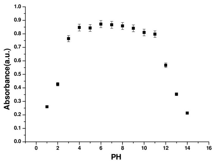
**Figure. S3** Effect of pH on the triazole-carboxyl Ag NPs solution
